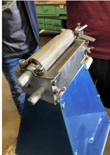
Figure 10. The modified barley mill was used to flake the whole kernels.
