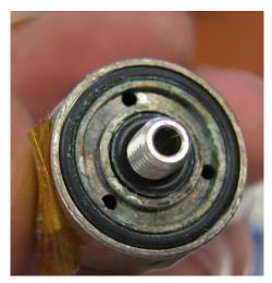
Figure 8.—Corrosion and residue on surface of 316 SS (stainless steel) solenoid valve used in H<sub>2</sub> vent service for fuel cell system.
