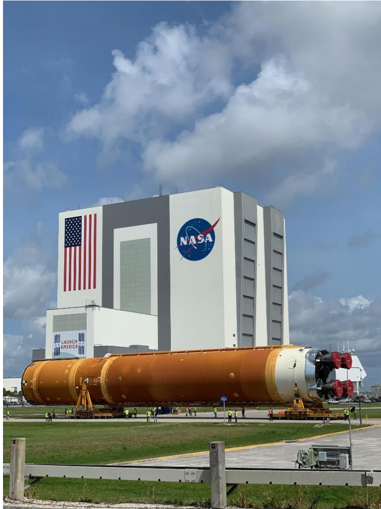
Fig. 7 The 212-foot SLS core stage is transported to the VAB in April.
