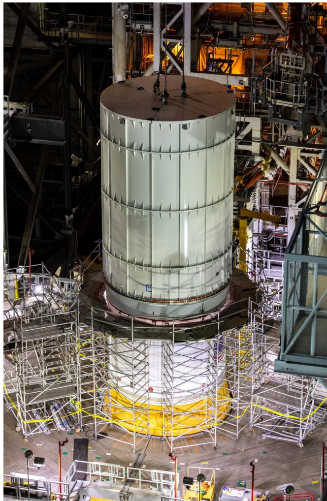
Fig. 5 The Orion mass simulator was stacked on the Artemis I rocket for modal testing on SLS prior to the Artemis I launch.
