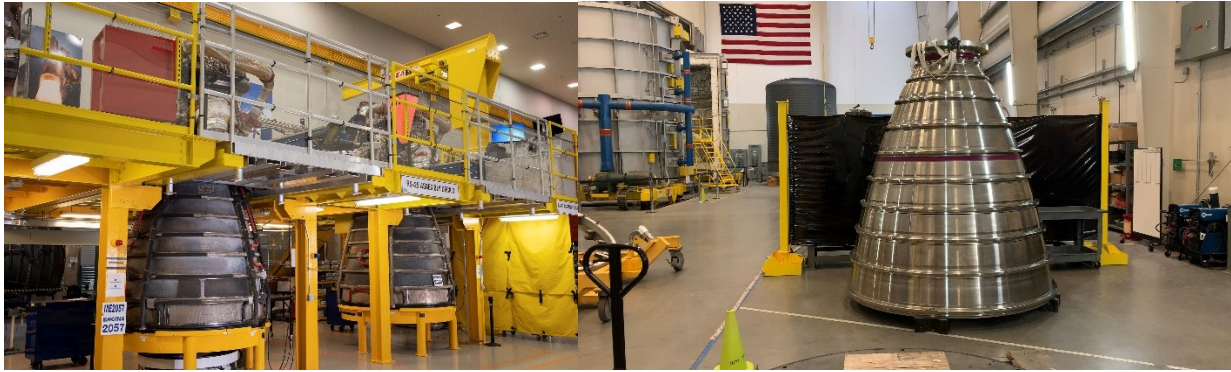
Fig. 10 Two RS-25 engines for the Artemis III mission undergo inspection at SSC, left, and an RS-25 nozzle from the new production line for Artemis V and beyond, right.
