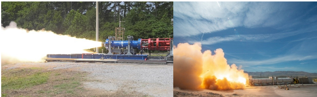
Fig. 13 A subscale solid rocket motor test, left, at MSFC supports the evolved boosters, while a full-scale SRB test Utah, right, evaluates potential new materials and processes for missions beyond Artemis III.
