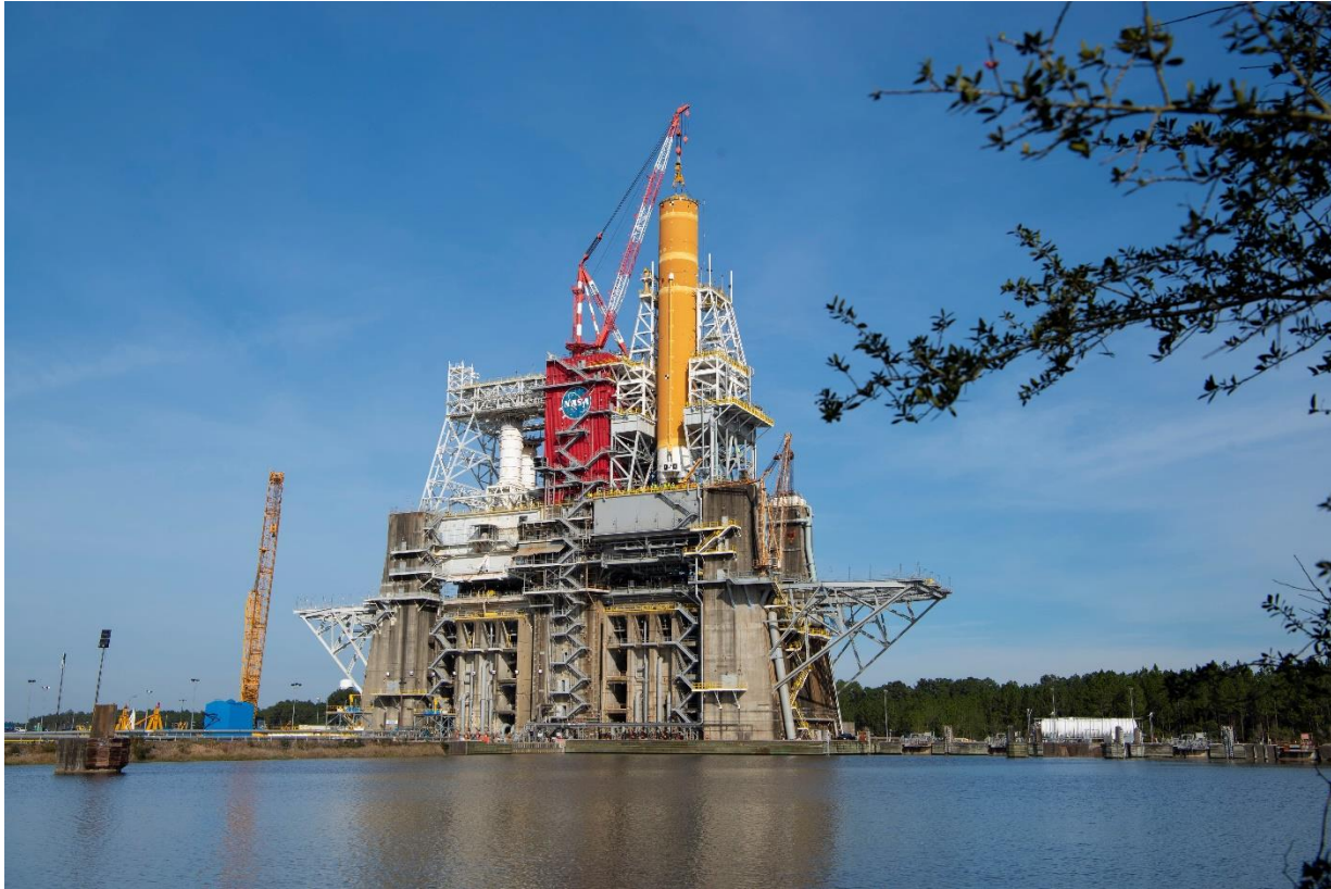
Figure 8. The SLS core stage is currently undergoing "green run" testing at Stennis Space Center (SSC) in preparation for the Artemis I flight.
