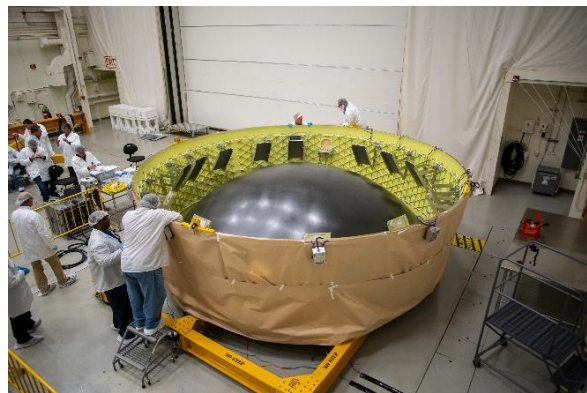
Figure 9. The completed Orion Stage Adapter (OSA) with brackets to hold the 13 6U CubeSats in dispensers (and avionics unit) that are manifested on the Artemis I flight.
