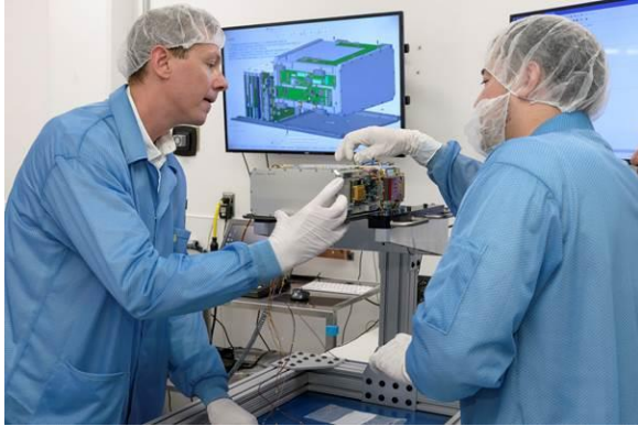
Figure 6. Team members assemble the BioSentinel spacecraft, which will study the effects of radiation on yeast in deep space.
