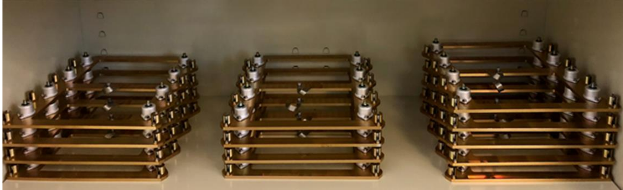
Figure 7. Vibration mitigation system for Artemis I 6U CubeSats.
