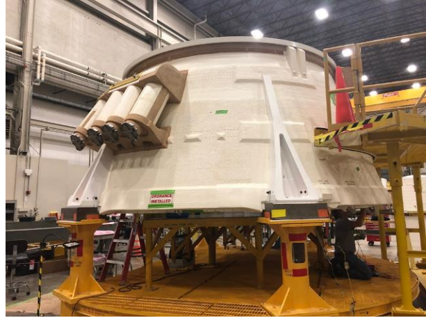
Figure 9. An aft skirt for the Artemis I solid rocket boosters is nearly complete at Kennedy Space Center (KSC). Four booster separation motors are visible.
