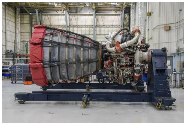
Figure 11. Completed RS-25 engine ready for installation in the Artemis I core stage.
