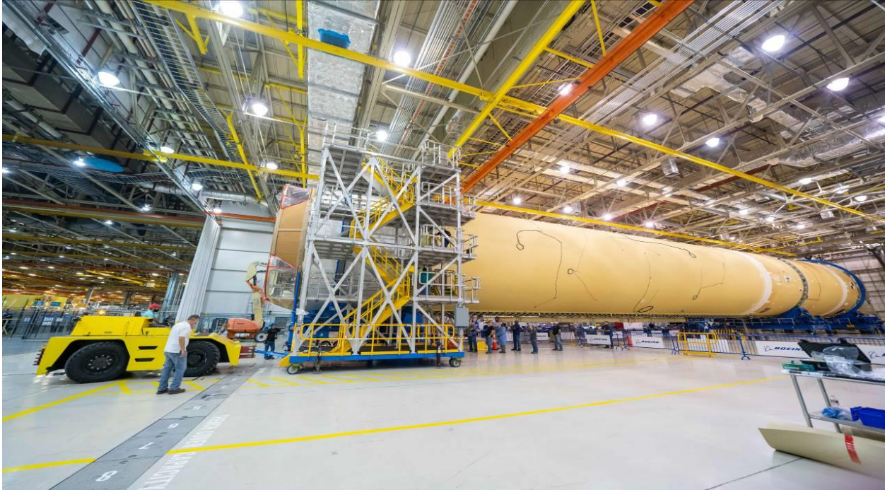
Figure 12. Technicians at Michoud Assembly Facility near New Orleans have structurally joined the SLS Core stage for the Artemis I flight.
