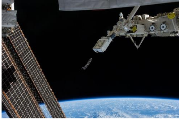
Figure 1 Flock 1 is a constellation of CubeSats dedicated to Earth Observations achieving resolutions of three to five meters. 2
