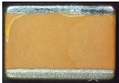
e) Cracking caused by manual soldering.
