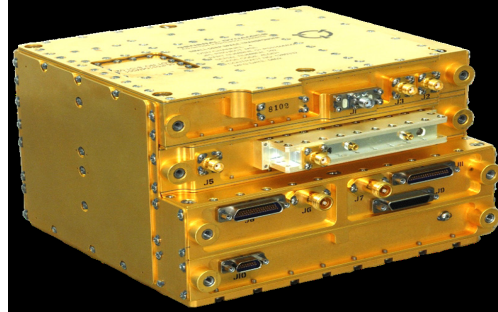
Figure 5.4—Image of Representative SDST communications hardware.
