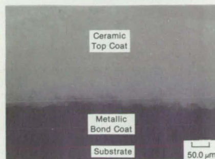
INFILTRATED WITH FLUORESCENT EPOXY
