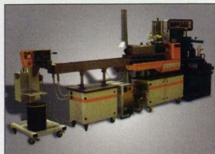
Figure 3: LPKF system: Heating-cooling mixer combination, extruder, cooler, and granulator at FH Lippe (from right to left)
