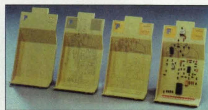
Figure 4: Complete chain for manufacturing a 3D-MID: molding, activation, plating, and component assembly
