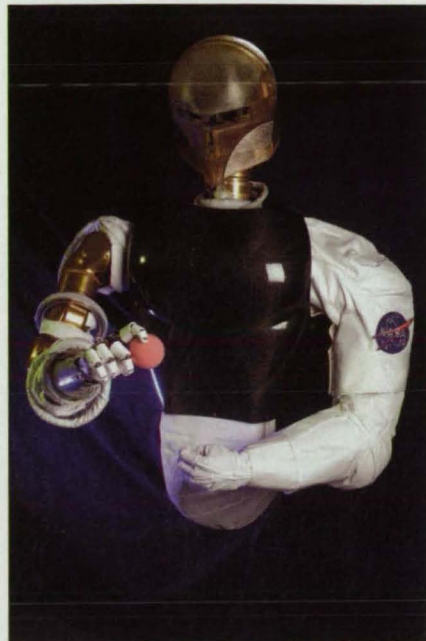
NASA's Robonaut features advanced mechatronics, including more than 150 sensors per arm. (Photo courtesy of NASA)
