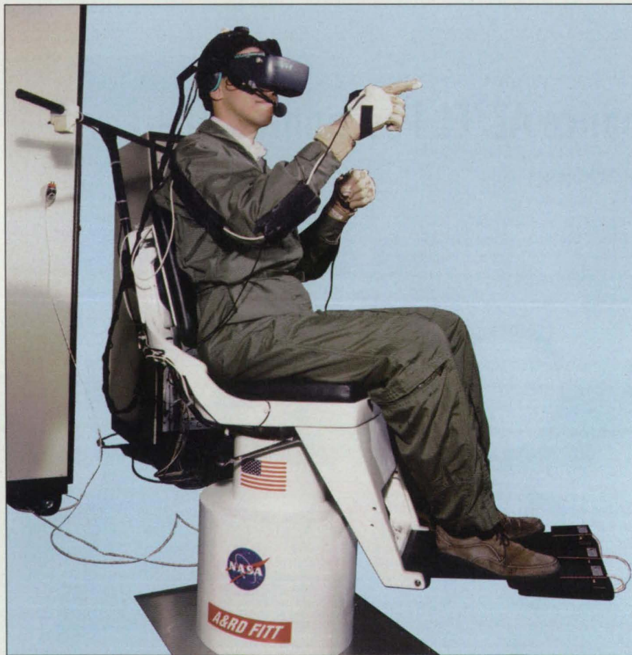
An Operator Using the FITT controls a remote robot by a combination of hand, arm, head, and foot motions and vocal commands.
