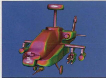
Surface pressure contours on an Apache-Longbow attack helicopter computed with Cart3D simulation software.
