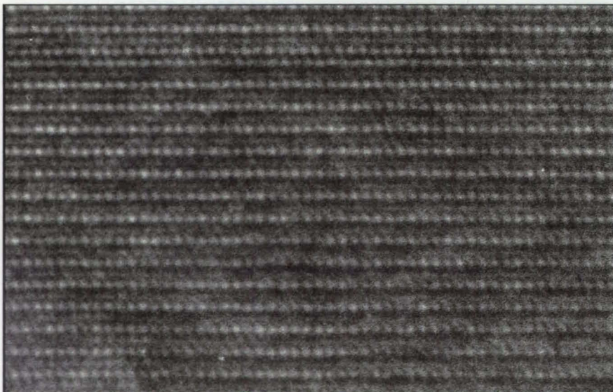
This Electron Micrograph shows two 2H SiC columnar grains and the interface between them. Except for a few faults (especially near the top) wherein small regions have the 3C structure, the grains are relatively free of defects. Notice that at the interface between the grains, the basal planes are nearly continuous.
