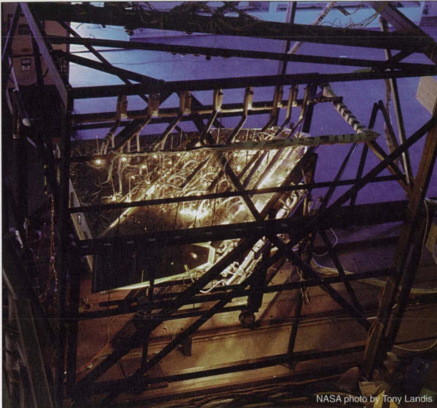
Figure 2. The Radiant Heater Is Shown in Use in a radiant-heating test. The heater produced heat fluxes up to 30 Btu/(ft 2 ·s) (3.4 × 10 5 W/m 2 ) in the most brightly lit areas.
