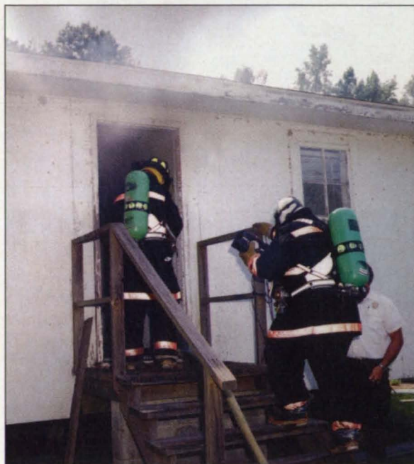
Stennis Space Center's fire department set fire to an abandoned building on-site to demonstrate how the FIRESCAPE fire imager also works on visible fires, in addition to "seeing" invisible flames of hydrogen and alcohol. Here, an SSC fireman uses the handheld imager to see through dense smoke to find a "victim" trapped in the building.
