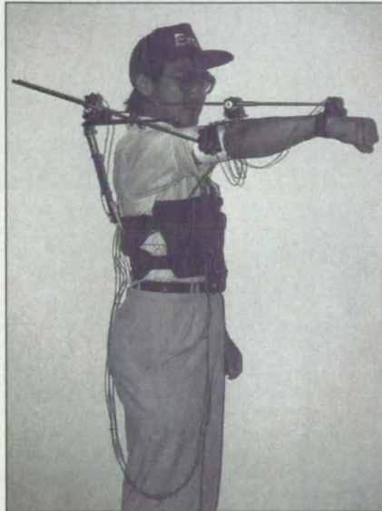
Figure 1. The Exoskeletal Apparatus is strapped to the wearer for measuring arm motions.
