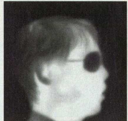
Figure 2. This is One Frame from a video image obtained with a 15- \mu\text{m} wavelength QWIP. NE\Delta T = 30 mK.
