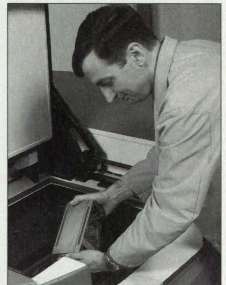
Figure 2. The operator loads the Test Fixture containing the unit under test into one of the six test positions on the rotor.
