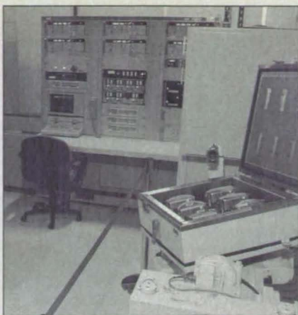
Figure 3. The Tester Control Room houses the consoles for controlling the centrifuge, the indexer (shown at the right of the photo), and the stimulus to the unit under test.
