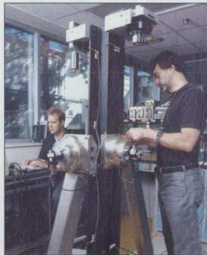
Marshall researchers Dr. Michael E. Polites (right) and Dean C. Alhorn perform a full-scale laboratory experiment for testing rotating unbalanced-mass (RUM) devices for scanning gimballed payloads and free-flying spacecraft.
