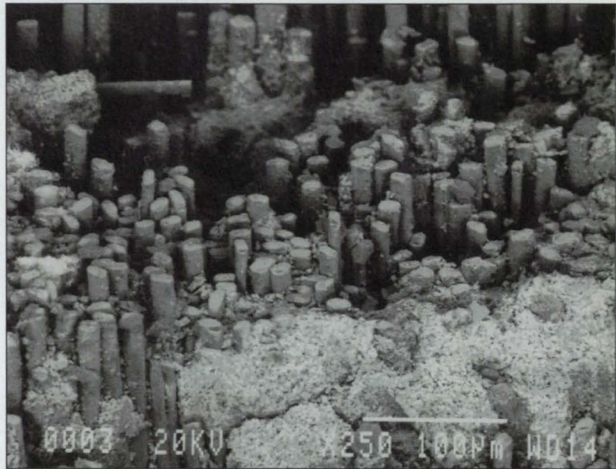
This Scanning Electron Micrograph shows a fracture surface of a specimen of glass-ceramic matrix composite material. Note that fibers have been pulled out: this is characteristic of a tough composite.
