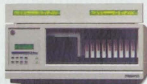
Our CY-8510A features one or two tape drives and can store up to 385 GB on eleven tapes—without tape handling
