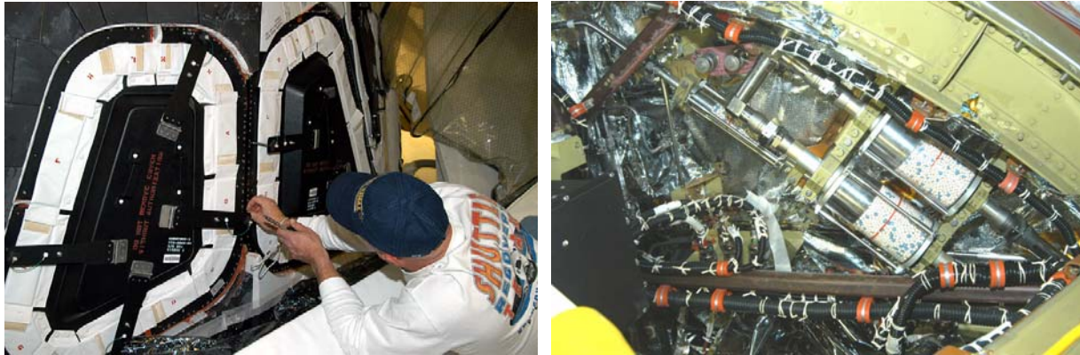
Figure 42. Design Requirements Force Frequent, Intrusive, and Labor-Intensive Window Cavity Conditioning System (WCCS) Filter/Desiccant Inspection and Replacement
