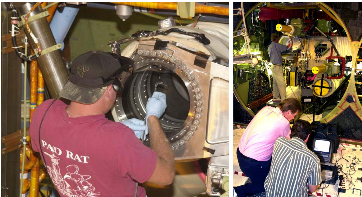
Figure 41. Technicians with Special Viewing Apparatus Use Fiber-Optics for Unplanned Inspections of Propulsion System Flow Liner on Orbiter Endeavour
