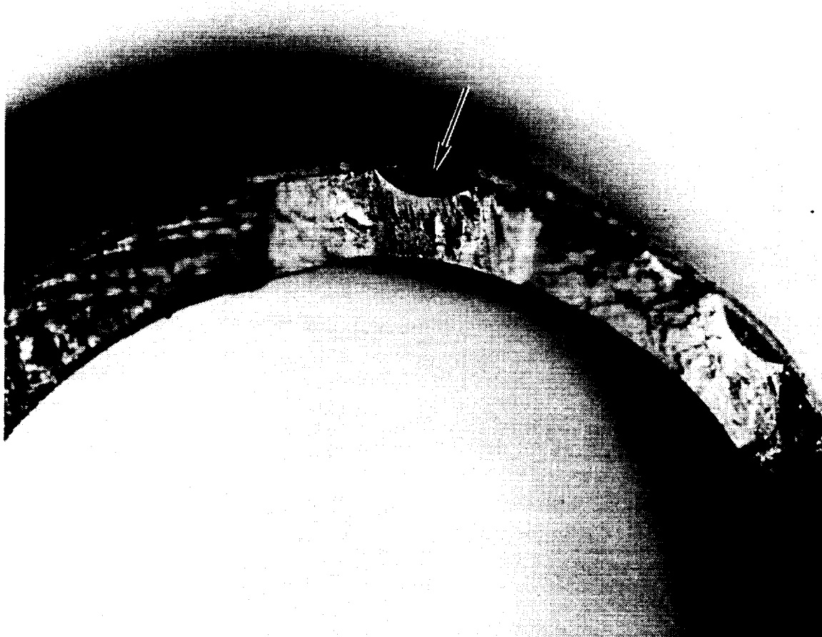
Figure 44 Optical Microscopy Image of PWA 286 Overlay Coated <213> PWA 1480 Specimen MB-17 After Out-of-Phase TMF Testing At 427-1038°C (800-1900°F), \pm 0.125\% , 1 cpm for 7294 Cycles. Arrow indicates typical coating initiated crack.
