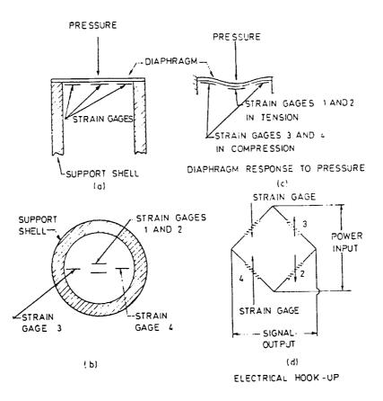
Figure 5 Silicon Based Semiconductor Strain Gauge Pressure Transducer
