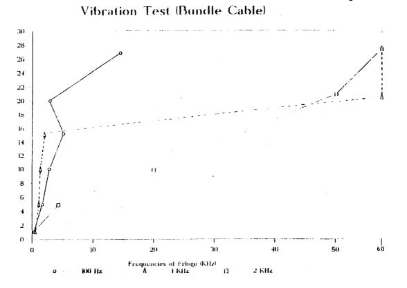
Visibility vs Cable Vibration Frequency
