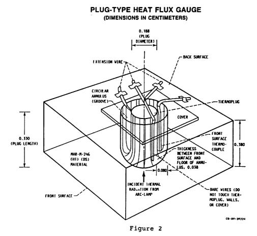
MINIATURE HEAT FLUX GAUGE BEFORE THERMOCOUPLE INSTALLATION
