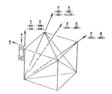
Figure 2. Notched specimen orientations that will be tested.
