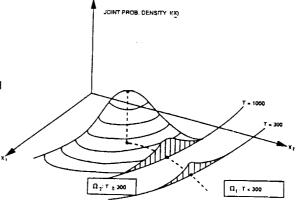
PROB. [ T < 300] =  $\int_{\Omega_1} \int f(X) X$  (PROB. OF FAILURE)
