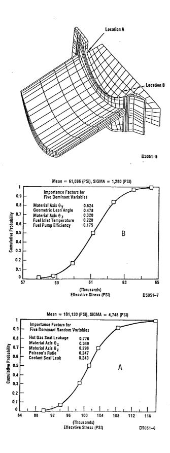
FIGURE 9. STRESS RESPONSE FOR HPFTP TURBINE BLADE
