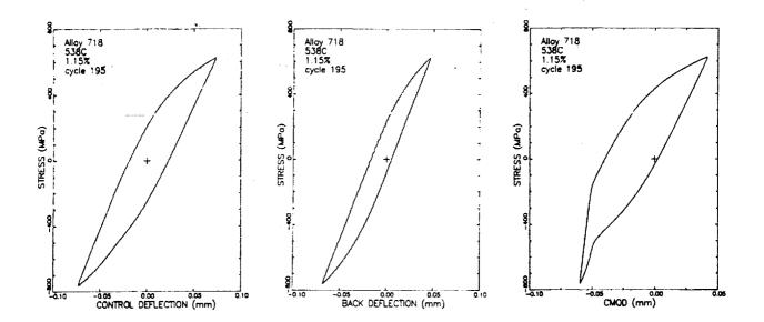
HYSTERESIS LOOPS FROM 538C ALLOY 718 TEST WITH A STRAIN RANGE OF 1.15% AND A MEAN STRESS OF ZERO
