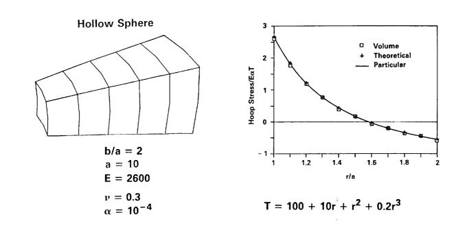
Temperature-Dependent Thermal Analysis Procedure Validated
