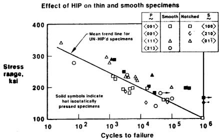
1200F PWA 1480 FATIGUE Effect of HIP on thin and smooth specimens
