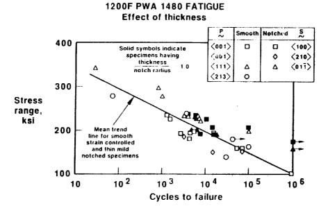
Figure 8. Thin, sharp notched and thick, mild notch specimens display a life trend different than the thin mild notch and smooth specimens.
