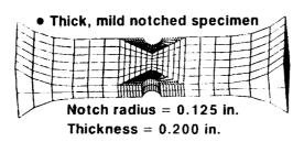
Figure 1. Notched fatigue specimen geometries and finite element meshes used to determine notch stresses.
