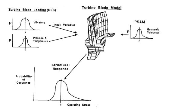
FIGURE 2. COMPONENT MODELS FOR LOADS AND STRUCTURAL ANALYSIS
