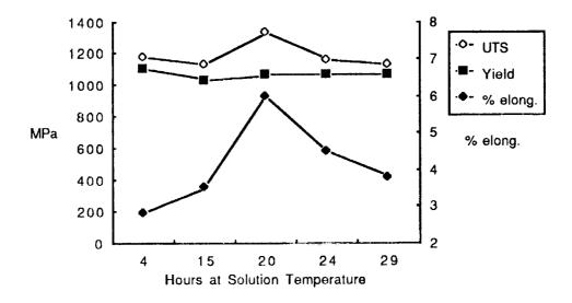
Figure 1. Effect of heat treatment solutionizing time on tensile properties. At 20 hours all of the eutectic  $\gamma$  is removed, and at longer times incipient melting becomes a factor. This shows that removing the eutectic  $\gamma$  can significantly increase ductility.
