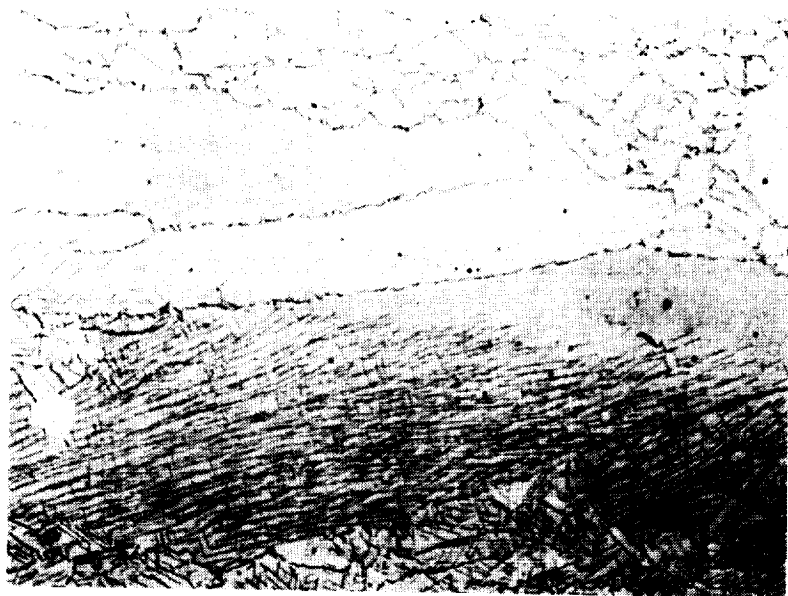
Figure 4 Alloy A With 3.93% Ti And 0.84% Al (Glyceria etch)
