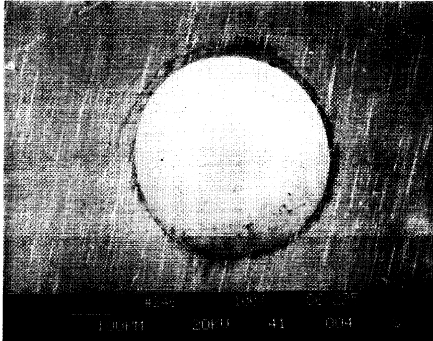
Figure 11: Half micron thick zirconium nitride, Rockwell "C" hardness indentation
