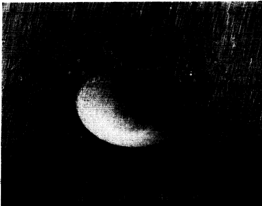
Figure 8: One micron thick molybdenum nitride coating, Rockwell "C" hardness indentation
