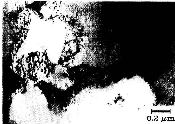
Figure 9. \gamma' by-pass and coarsening after tensile test to failure MAR-M 246, 1093 o C
