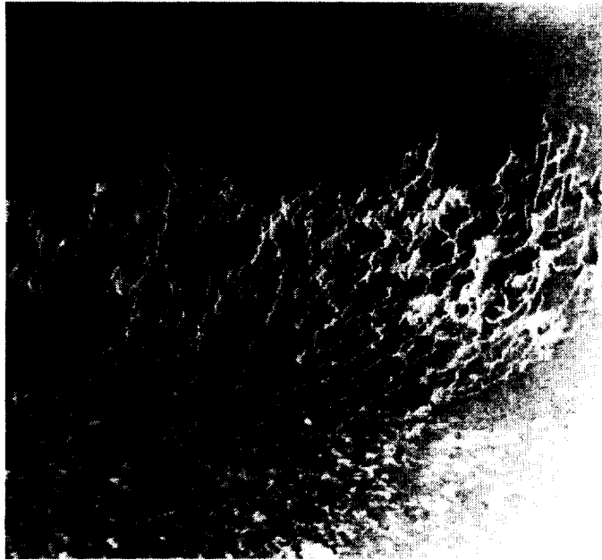
Fig. 12. Directional Orientation of Surface Distress Cracks on Ball
