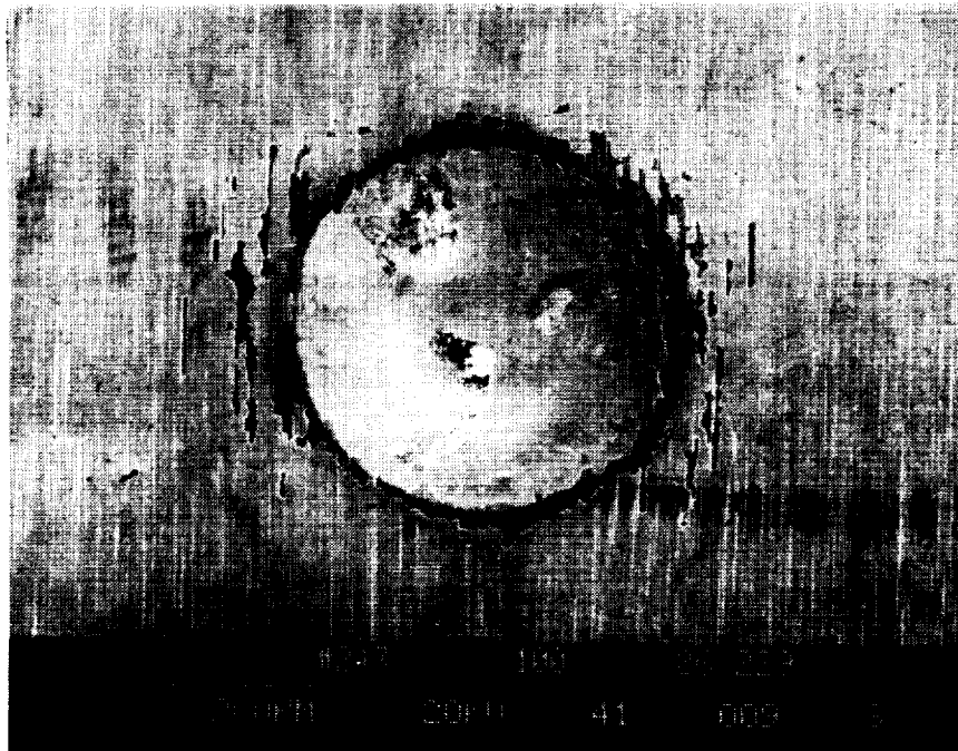
Figure 12: One micron thick zirconium nitride, Rockwell "C" hardness indentation
