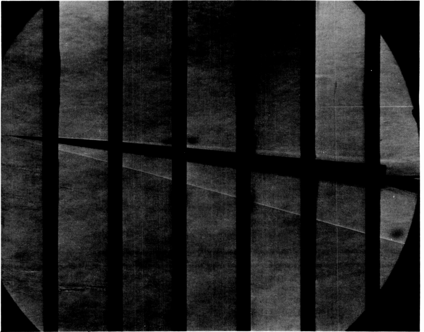
Figure 12. Shadowgraph of combined-theory wing model at M = 4.5 , R = 2.0 \times 10^6 per foot, and \alpha = 5.58^\circ .
