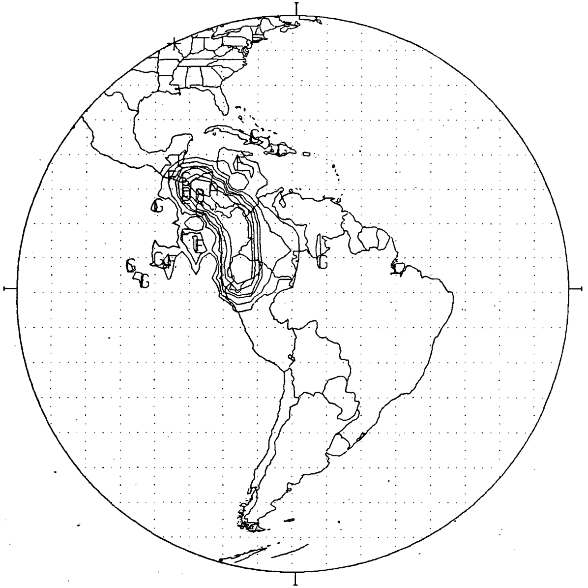
Figure 5.5.4-10 C-Band International Beam 6V Antenna Pattern
