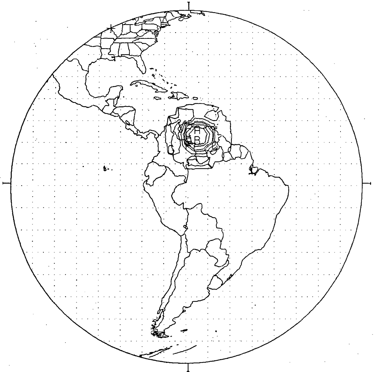
Figure 5.5.4-8 C-Band International Beam 4V Antenna Pattern
