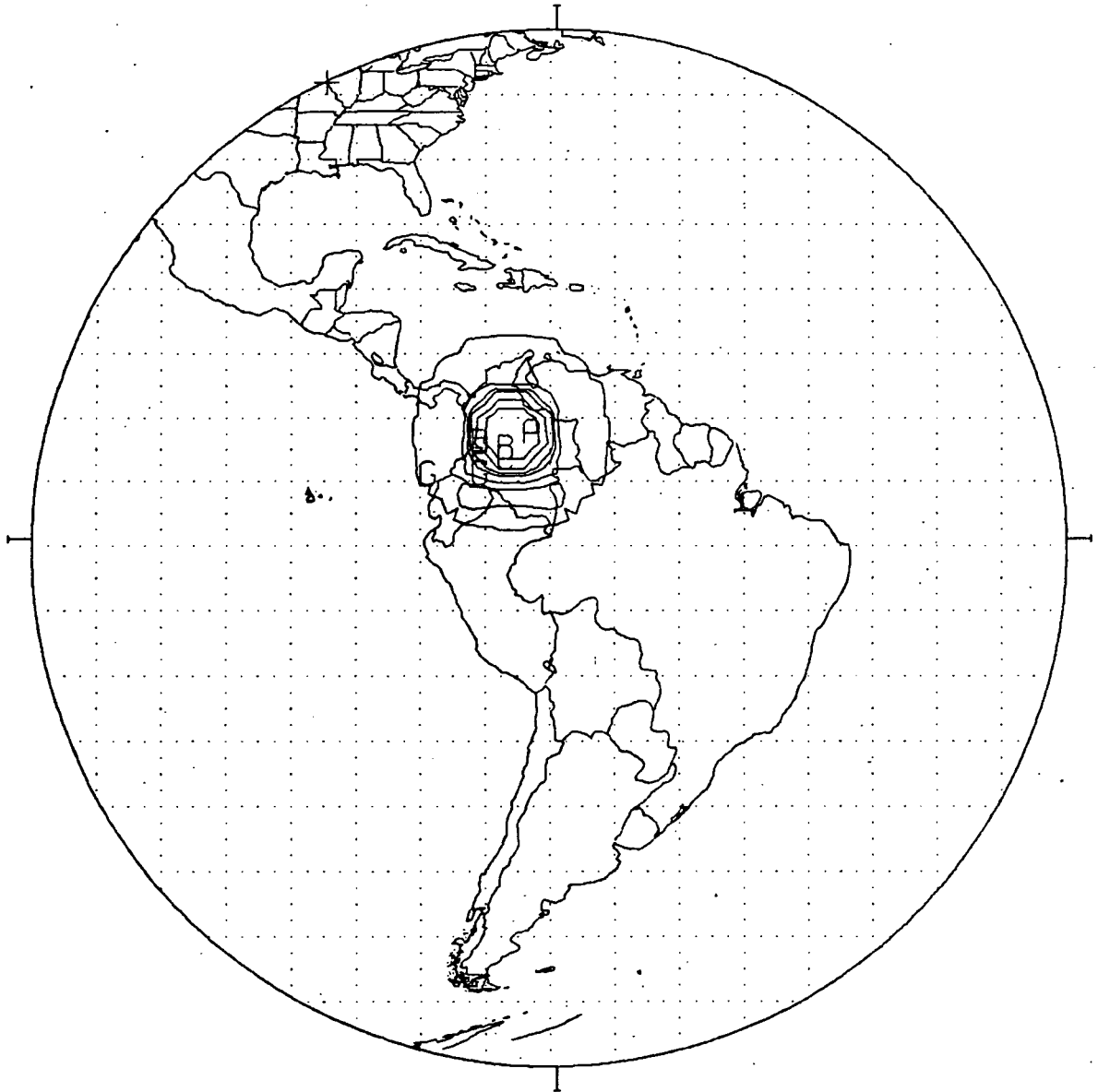
Figure 5.5.4-9 C-Band International Beam 5H Antenna Pattern
