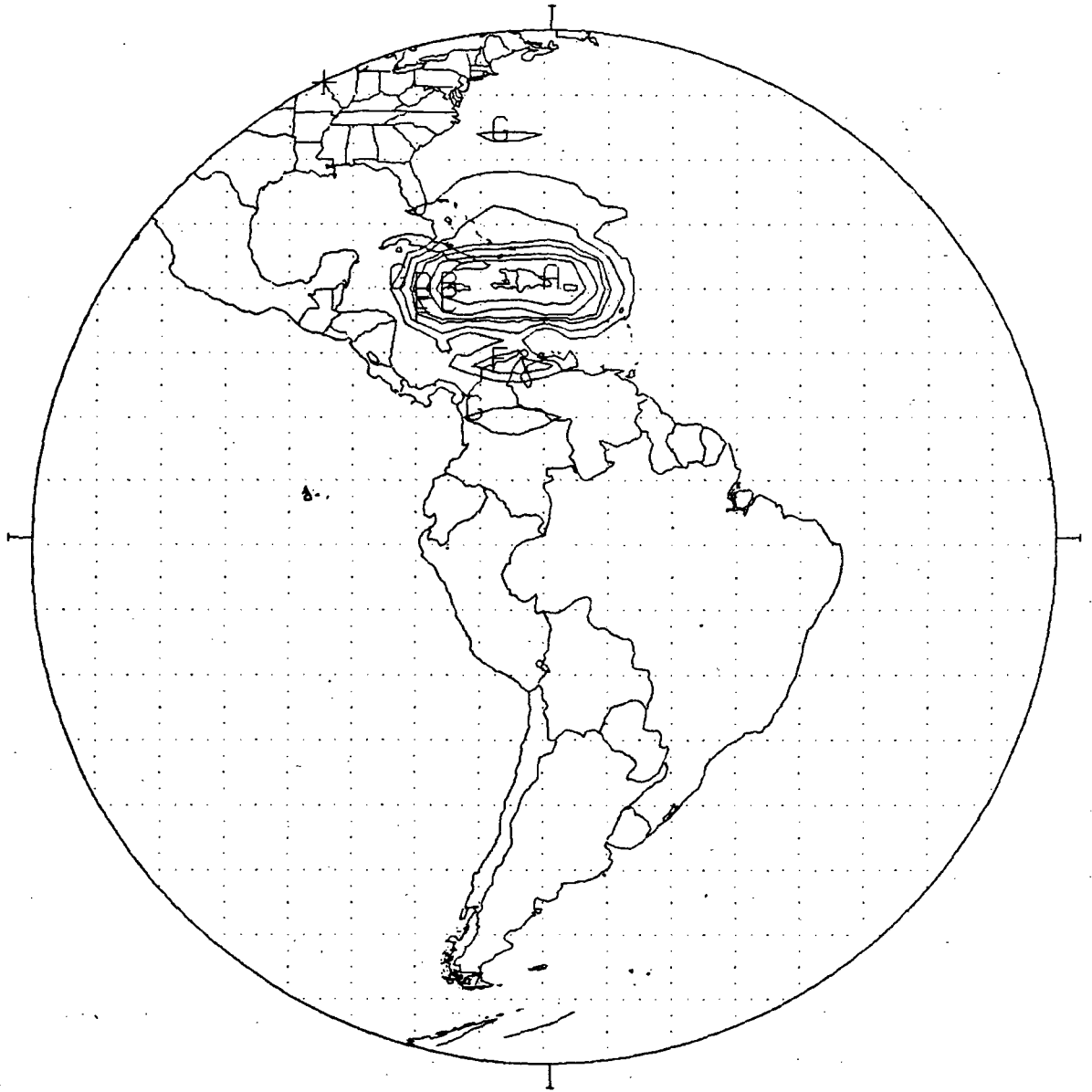
Figure 5.5.4-6 C-Band International Beam 2V Antenna Pattern
