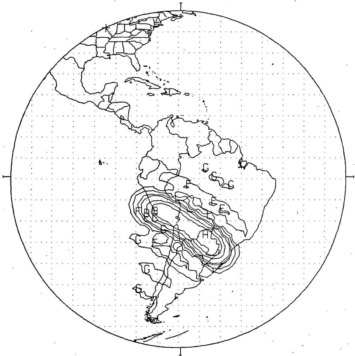
Figure 5.5.4-11 C-Band International Beam 7V Antenna Pattern
