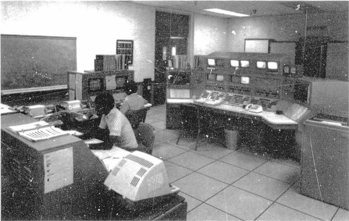
Fig. 2-5. Photograph of the Goldstone, California, 64-m antenna, Station 14 control console
