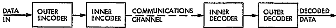
Fig. 2-7. Typical implementation of a concatenated coding scheme: outer encoder with block coding and inner encoder with convolutional coding.
