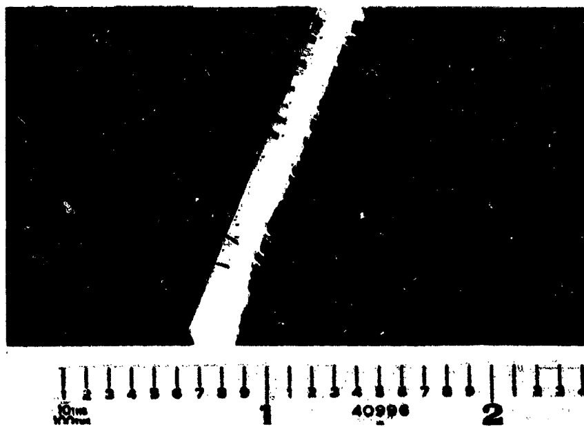
Figure 18. Typical Failure of a [\pm 67.5]_{82} Laminate
