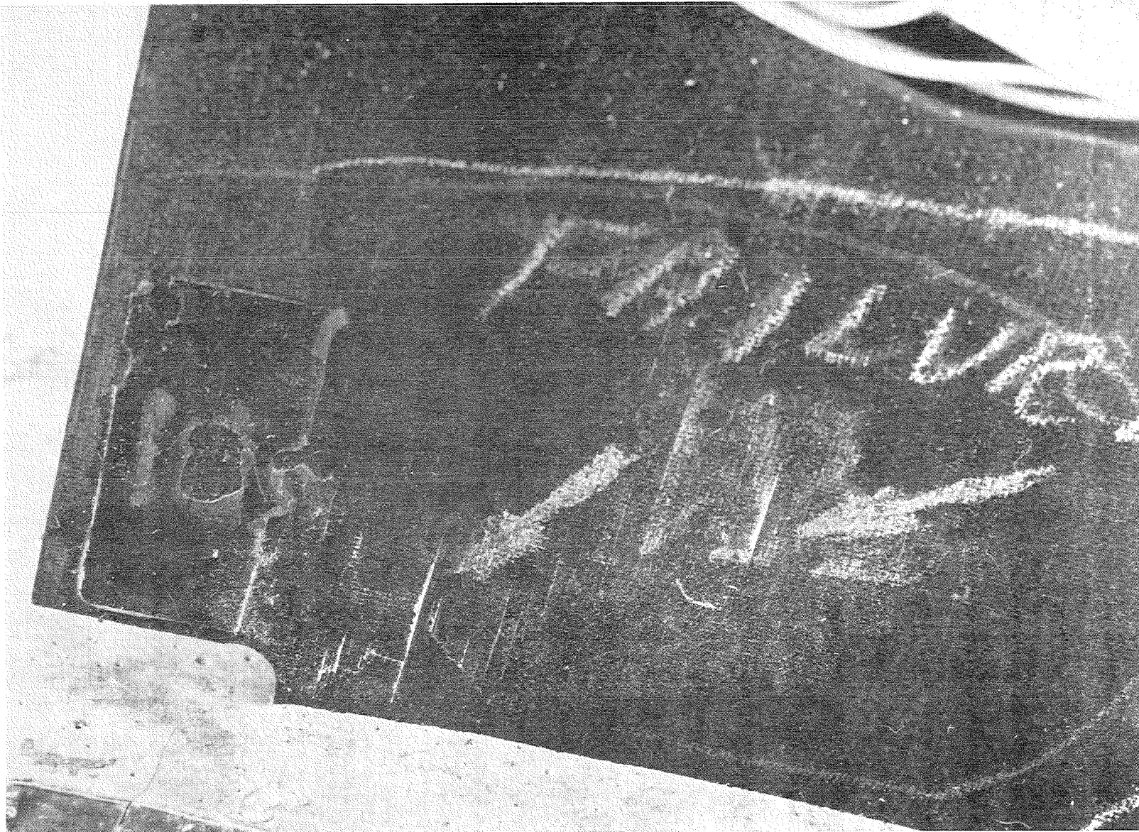
Figure 151. "Hat" Stringer Element EX109/EX110B Local Compression Failure, -132^{\circ}\text{C} ( -270^{\circ}\text{F} ) Test, Postcured.
