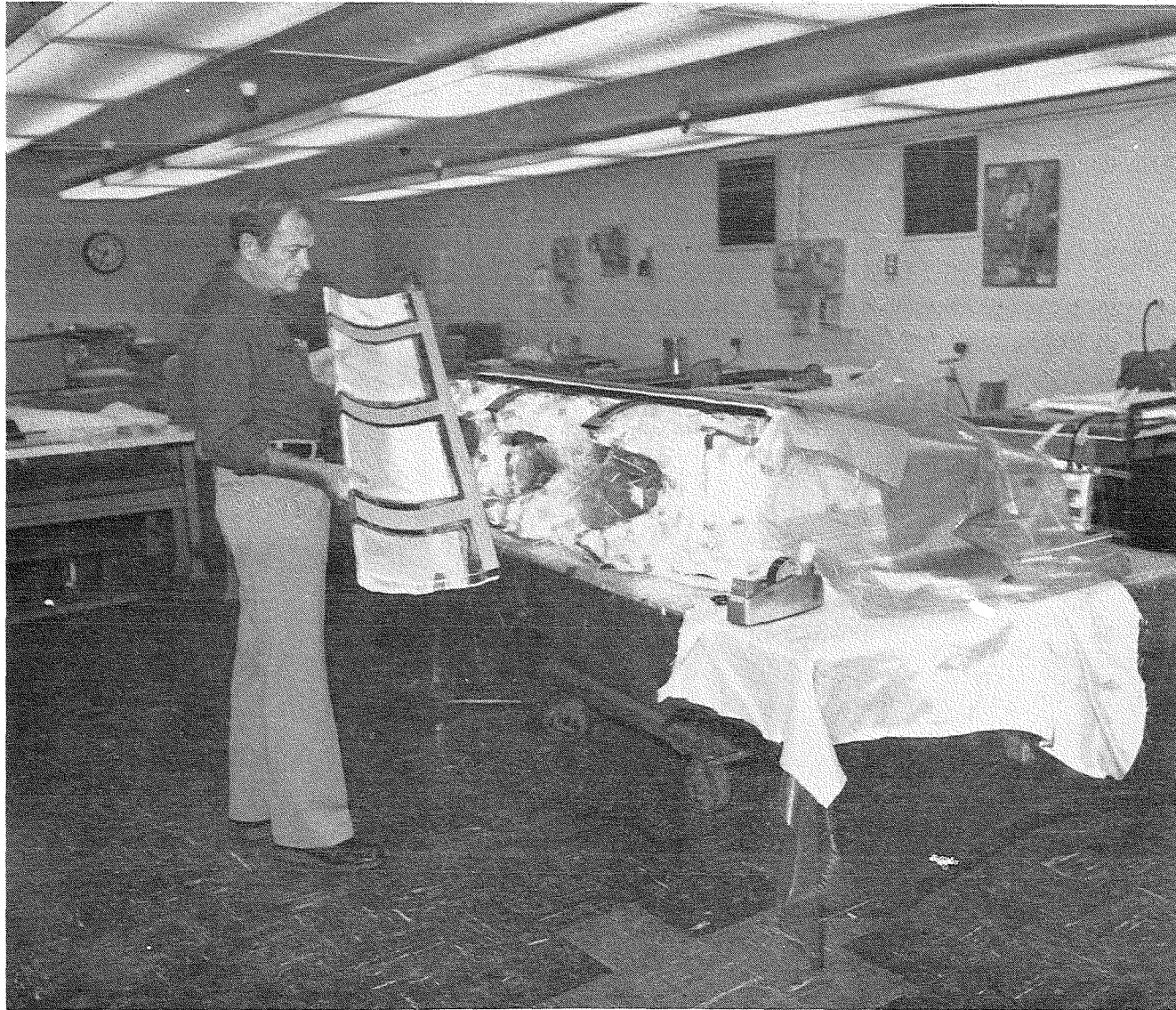
Figure 212. Lower Leading Edge Cover With Breather Material in Place
