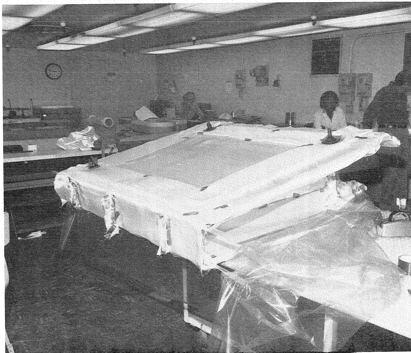
Figure 213. TDS With Lower Leading Edge Cover and Art Spar Installed and all Breather Material in Place
