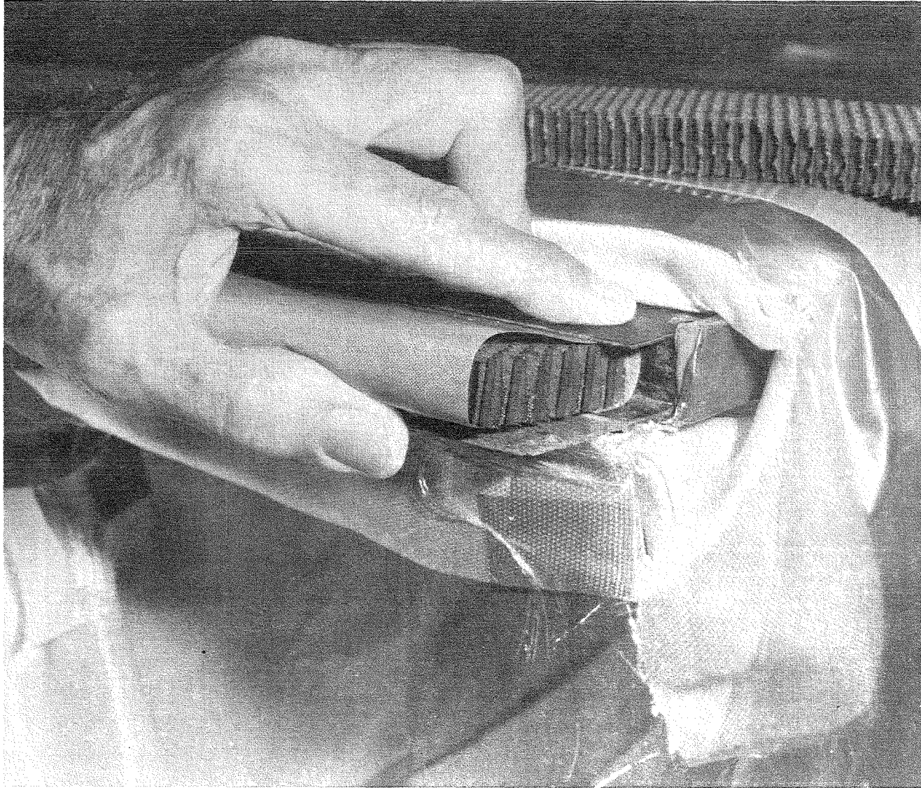
Figure 206. Honeycomb Inserted in TDS Cover Open Channel Closeout
