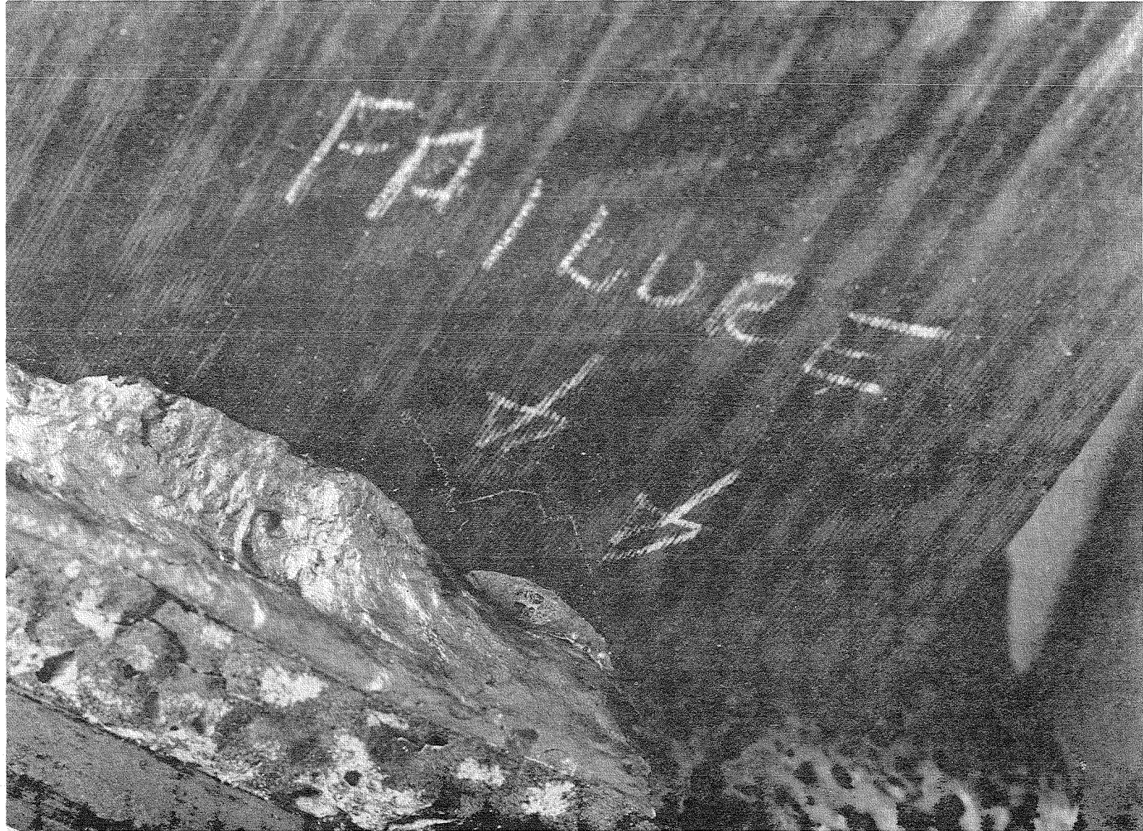
Figure 156. "I" Element EX194-1PC Showing Local Skin Compression Failure, 316 C (600 F) Test Postcured
