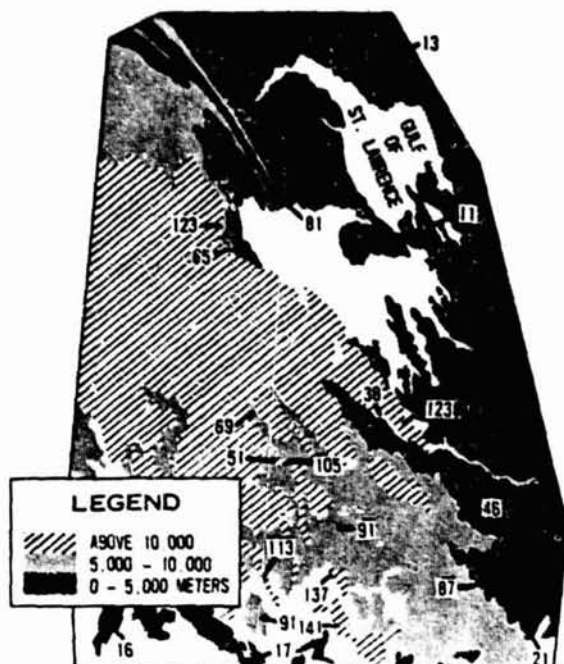
Fig. 2. Nova Scotia and surrounding areas including the stereographically measured heights (in hundreds of meters) of nearby clouds located as far as 67° of great-circle arc from the subsatellite point of the more remote satellite, SMS 2.
