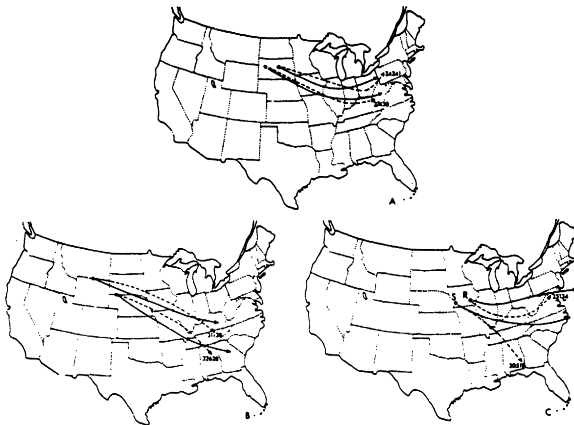
FIG. 4. Trajectories calculated using Danielsen's implicit scheme (solid) and using discrete model formulation (dashed) for period from 1200 GMT 10 May through 0000 GMT 11 May 1973. Final wind direction and speed are indicated for trajectories computed using discrete model formulation (27430 = 274° 30 m s -1 ).
