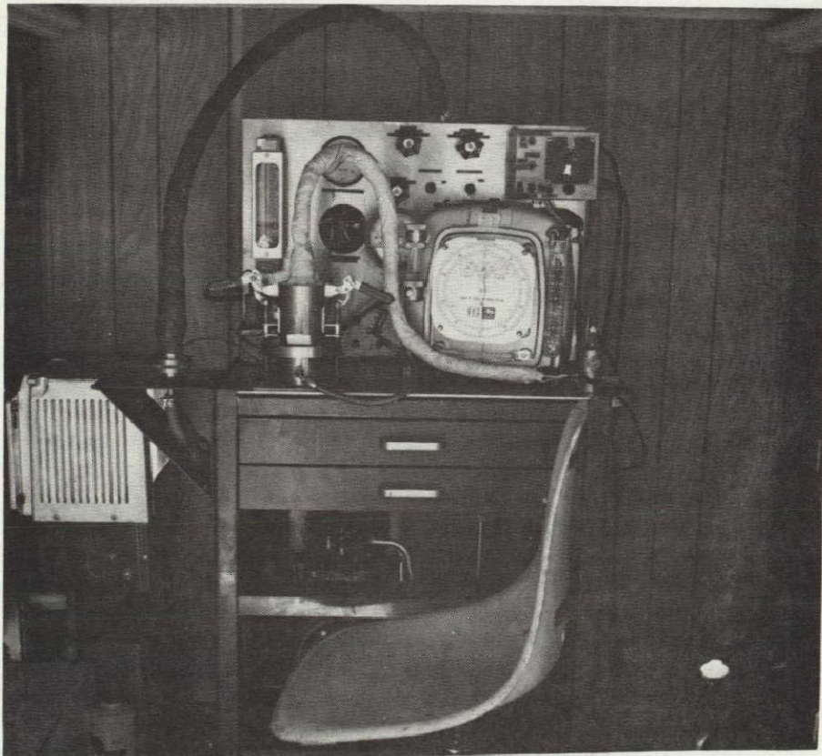
Figure 10. Mobile Smoke Analyzer.
