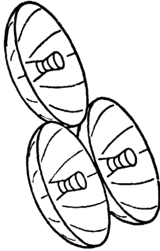
Figure 3-2 Deployable Parabolic Array
