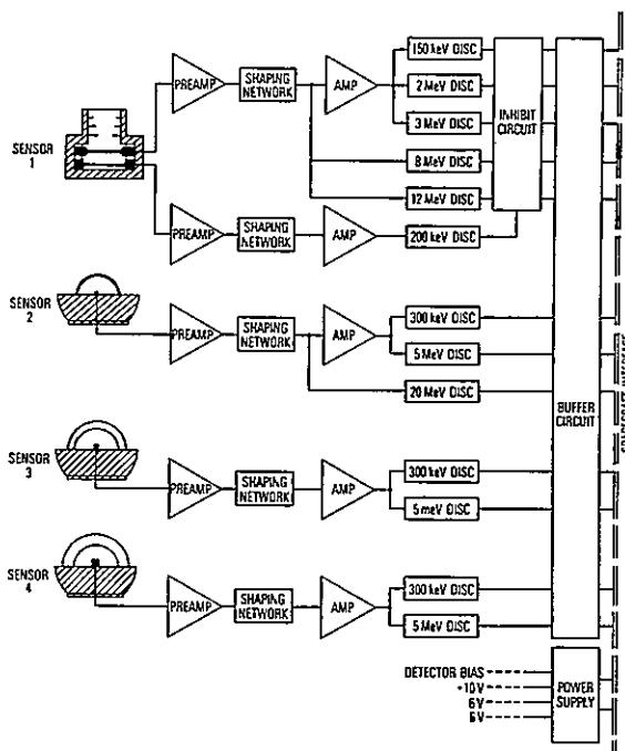
Fig 3 Schematic block diagram of detector/electronic system
