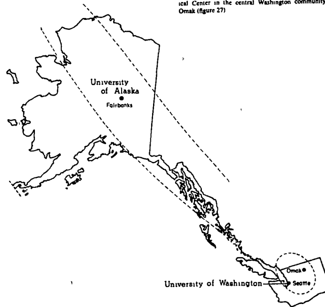
Figure 27 ATS-6 satellite footprints covering the three sites involved in the WAMI ATS-6 experiment. The difference in the area covered by each footprint (shown by dashed lines) reflects the difference in satellite look angles.
