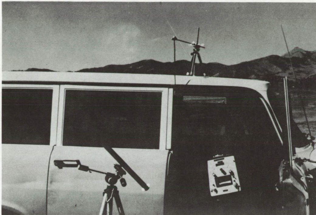
Figure 3. - Spectroradiometer field setup.
