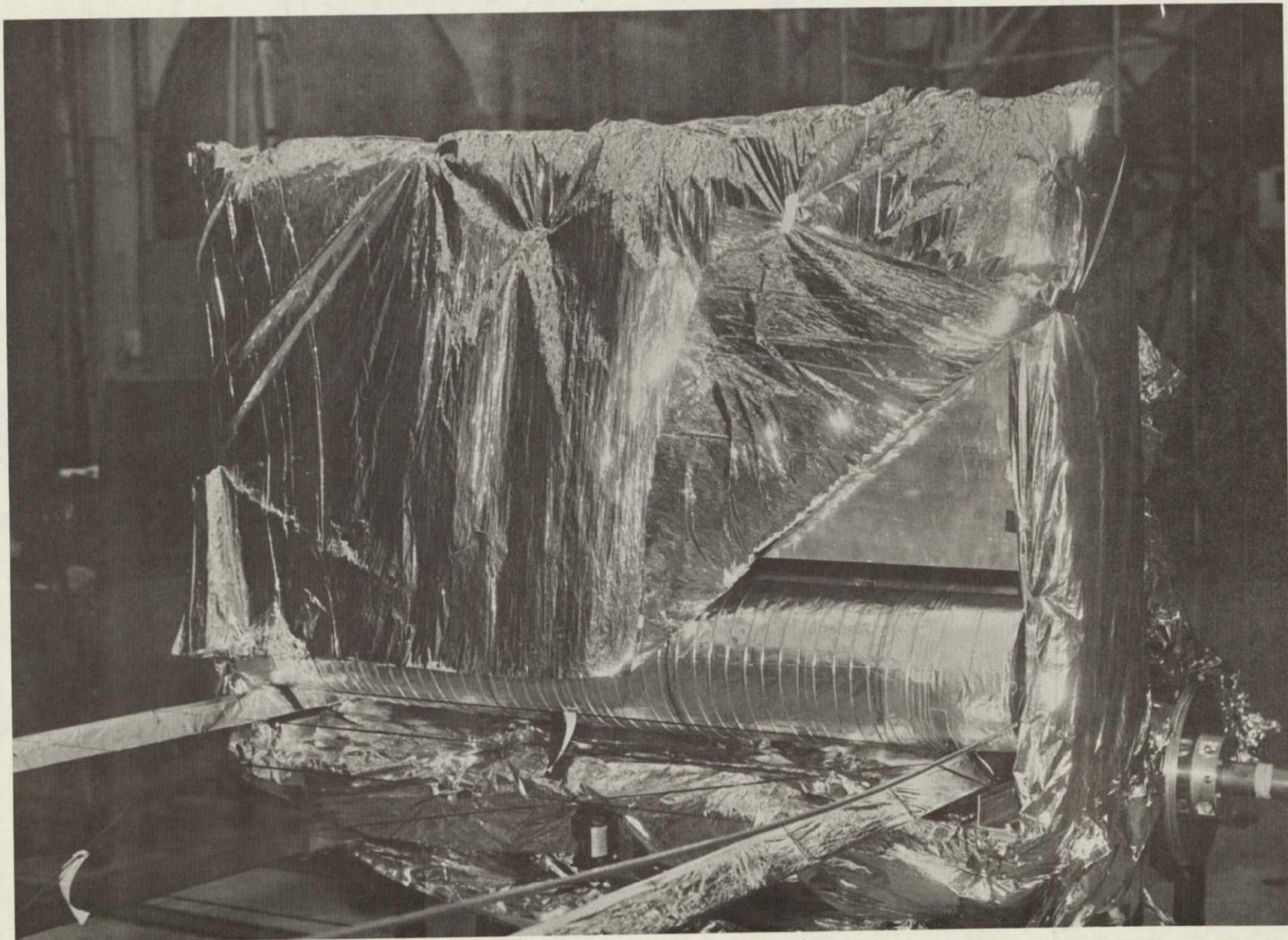
FIGURE 35 HARD TUBE FLEXIBLE RADIATOR TEST ARTICLE
