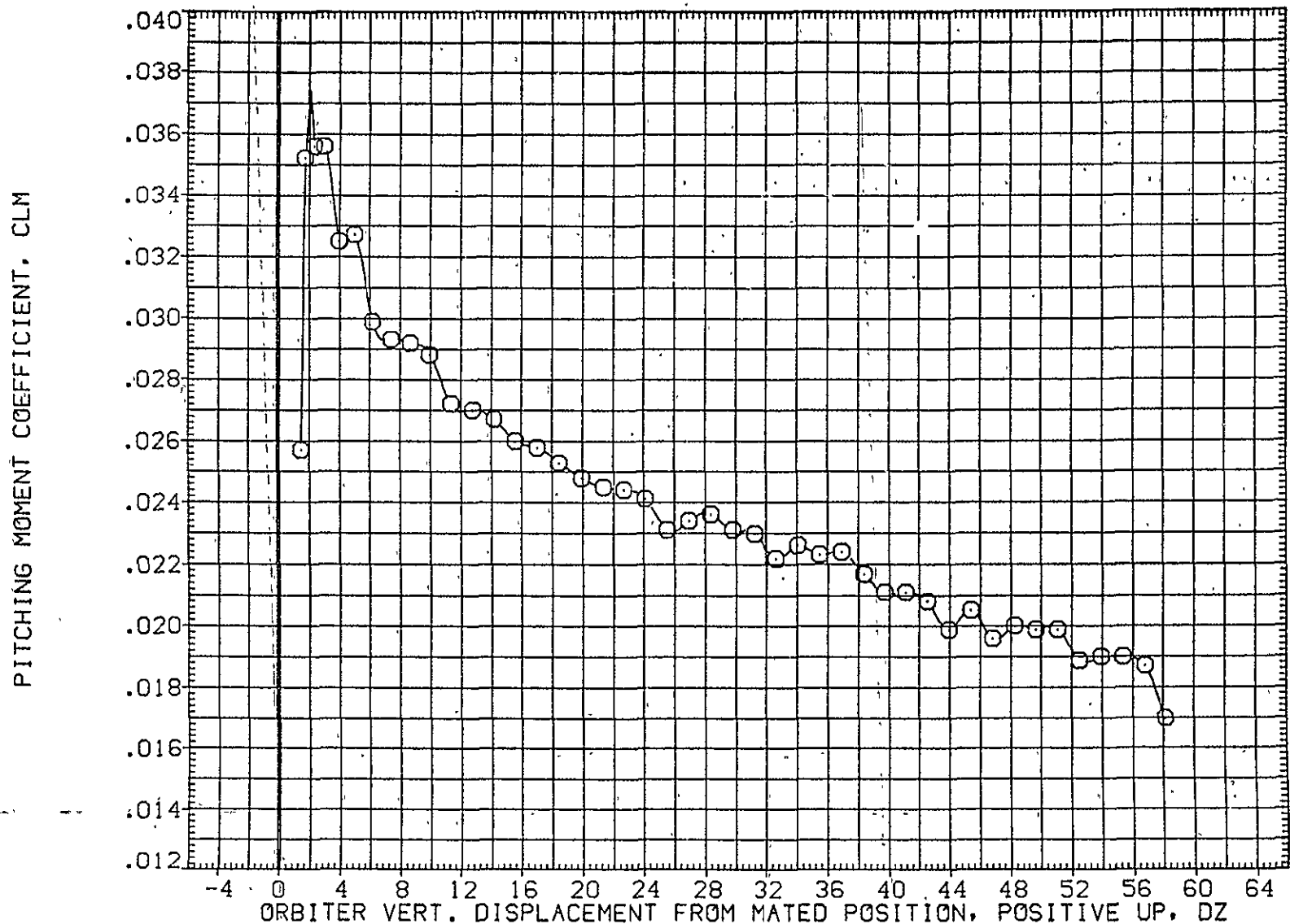
FIG. 38 ORB. DATA, CARRIER PROXIMITY, ALPHAC=2, IORB=8, BETAC=0, BETA0=0, AFE047
