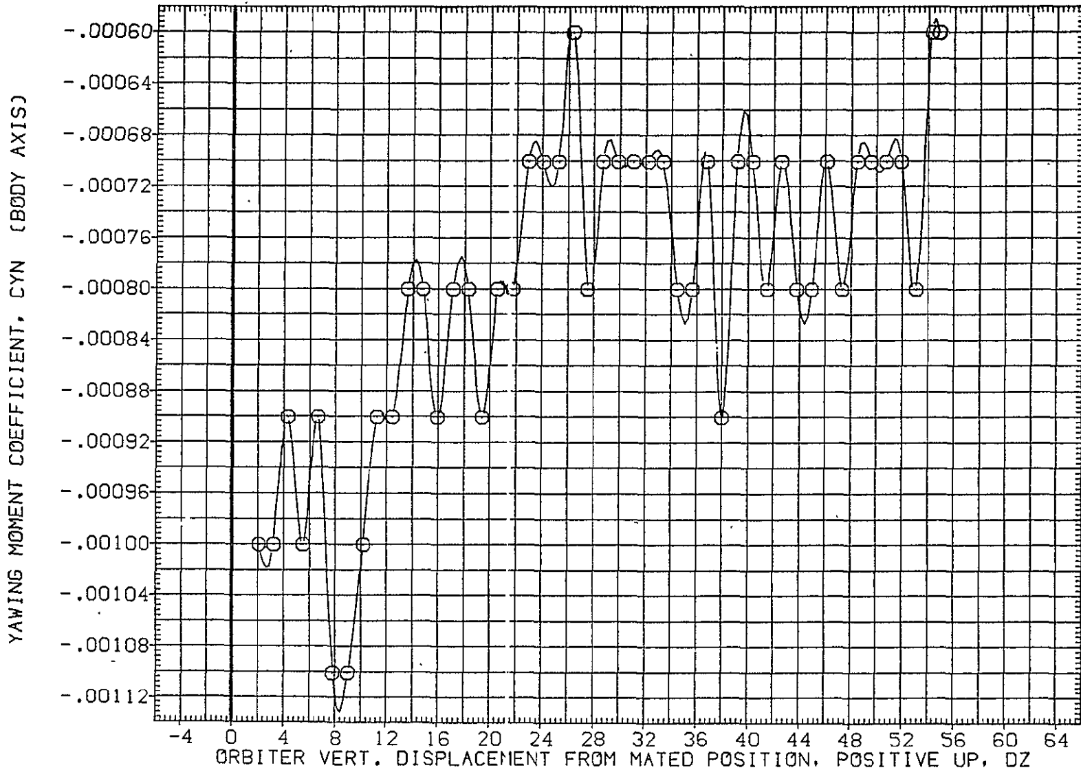
FIG. 25 ORB. DATA, CARRIER PROXIMITY, ALPHAC=0, IORB=6, BETAC=0, BETA0=0, AFE032
