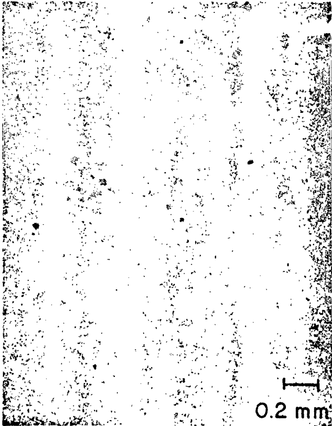
FIGURE 18A ENLARGED REGIONS OF SCANNER TOPOGRAPHS; HIGHLY PERFECT REGION
