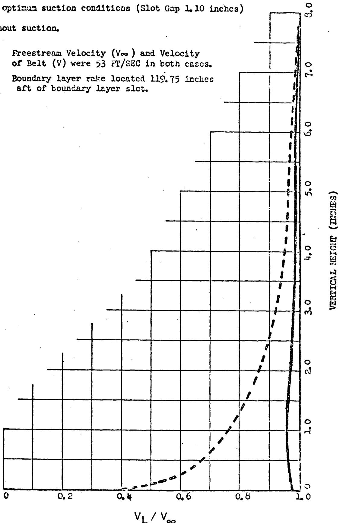
FIGURE 14 - MOVING GROUND BELT SURVEY-EFFECT OF BOUNDARY LAYER SUCTION
