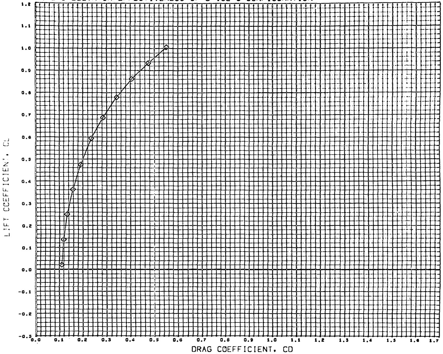
FIGURE-3 ELEVATOR EFFECTIVENESS OF B-18E-3 CONFIGURATION
