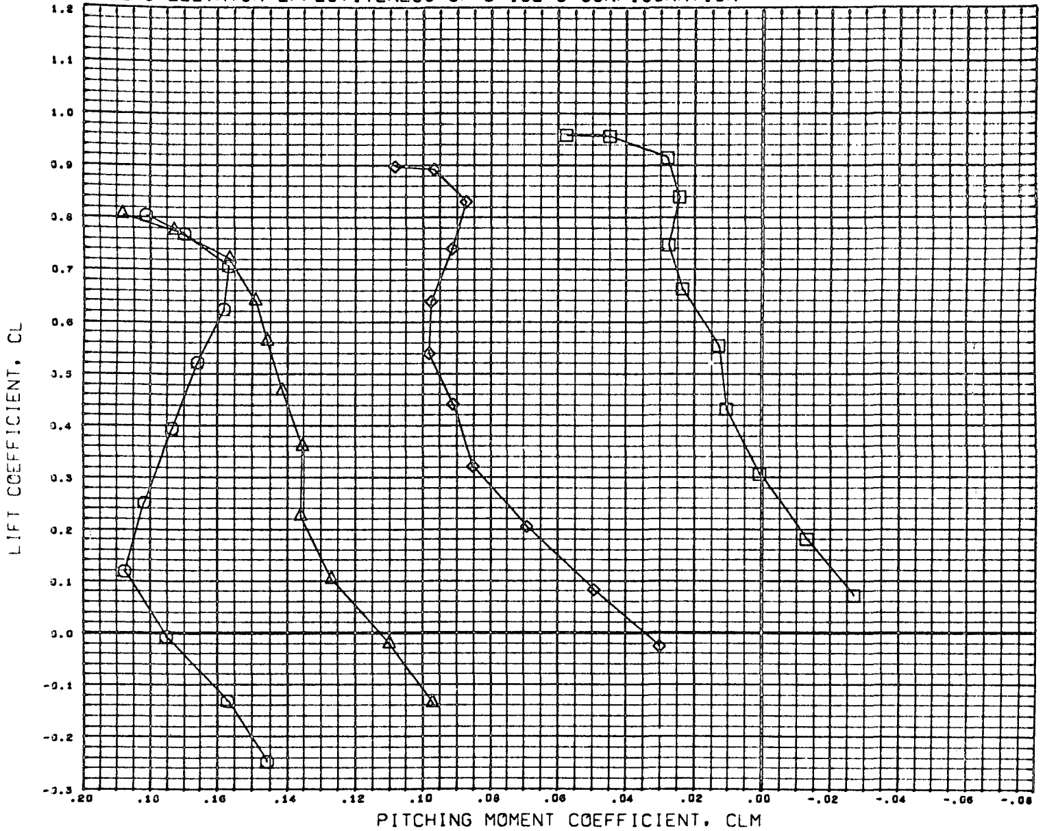
FIGURE-3 ELEVATOR EFFECTIVENESS OF B-18E-3 CONFIGURATION
