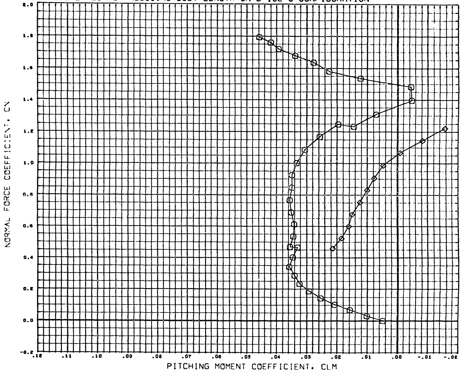
FIGURE-6 EFFECT OF REDUCING BODY LENGTH ON B-18E-3 CONFIGURATION
