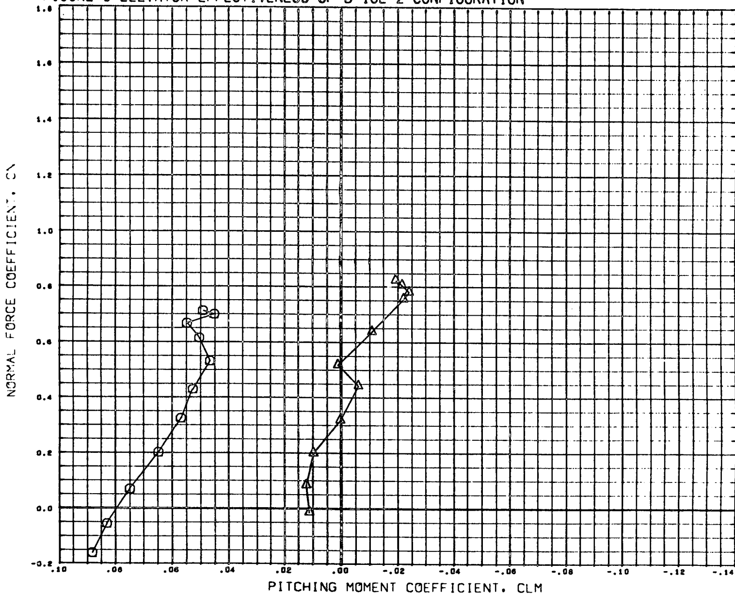
FIGURE-9 ELEVATOR EFFECTIVENESS OF B-18E-2 CONFIGURATION
