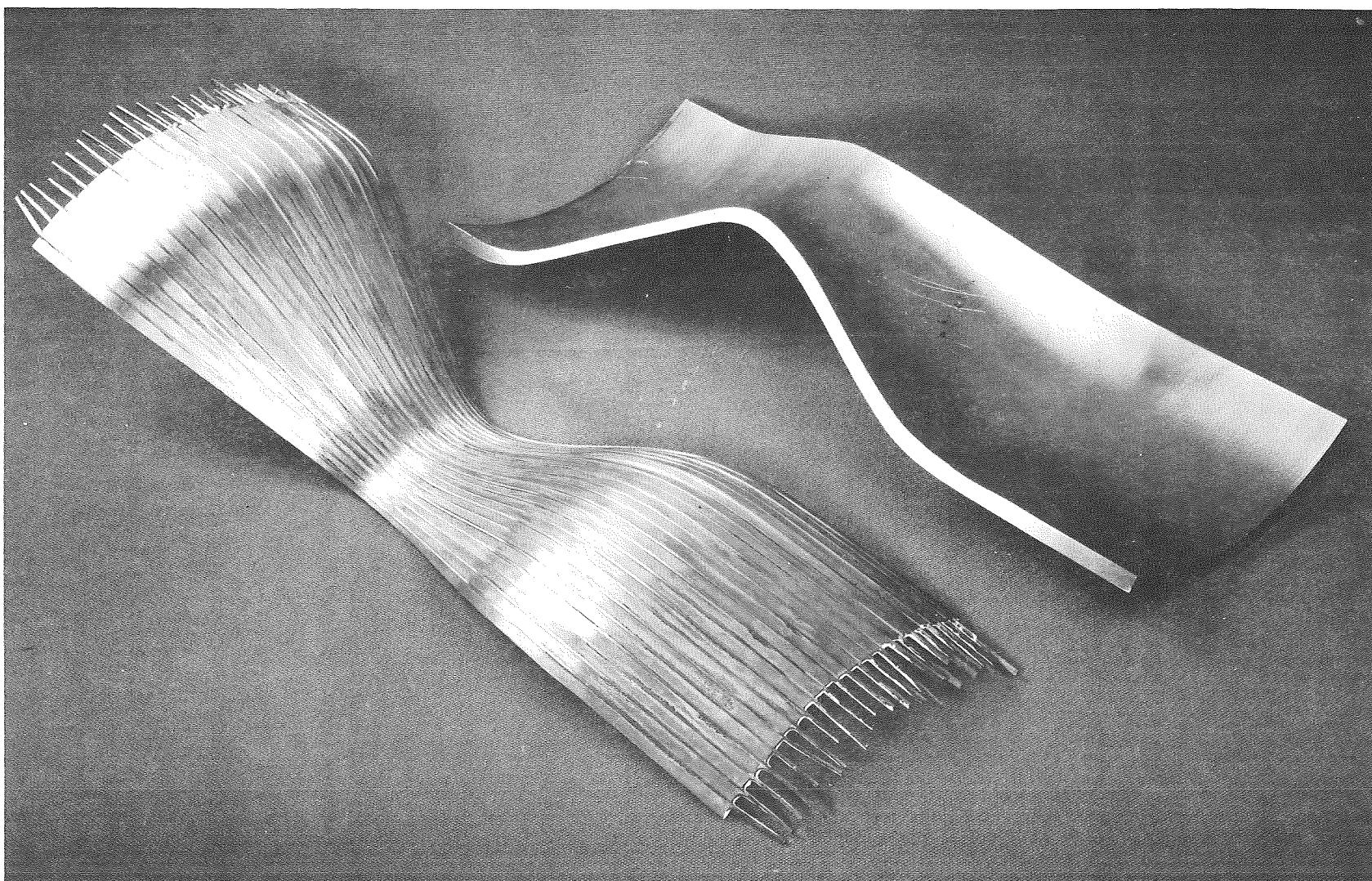
FIGURE 50. RIB-TOOLING AND SHELL COMPONENTS FOR NOZZLE WELDING EXPERIMENT
