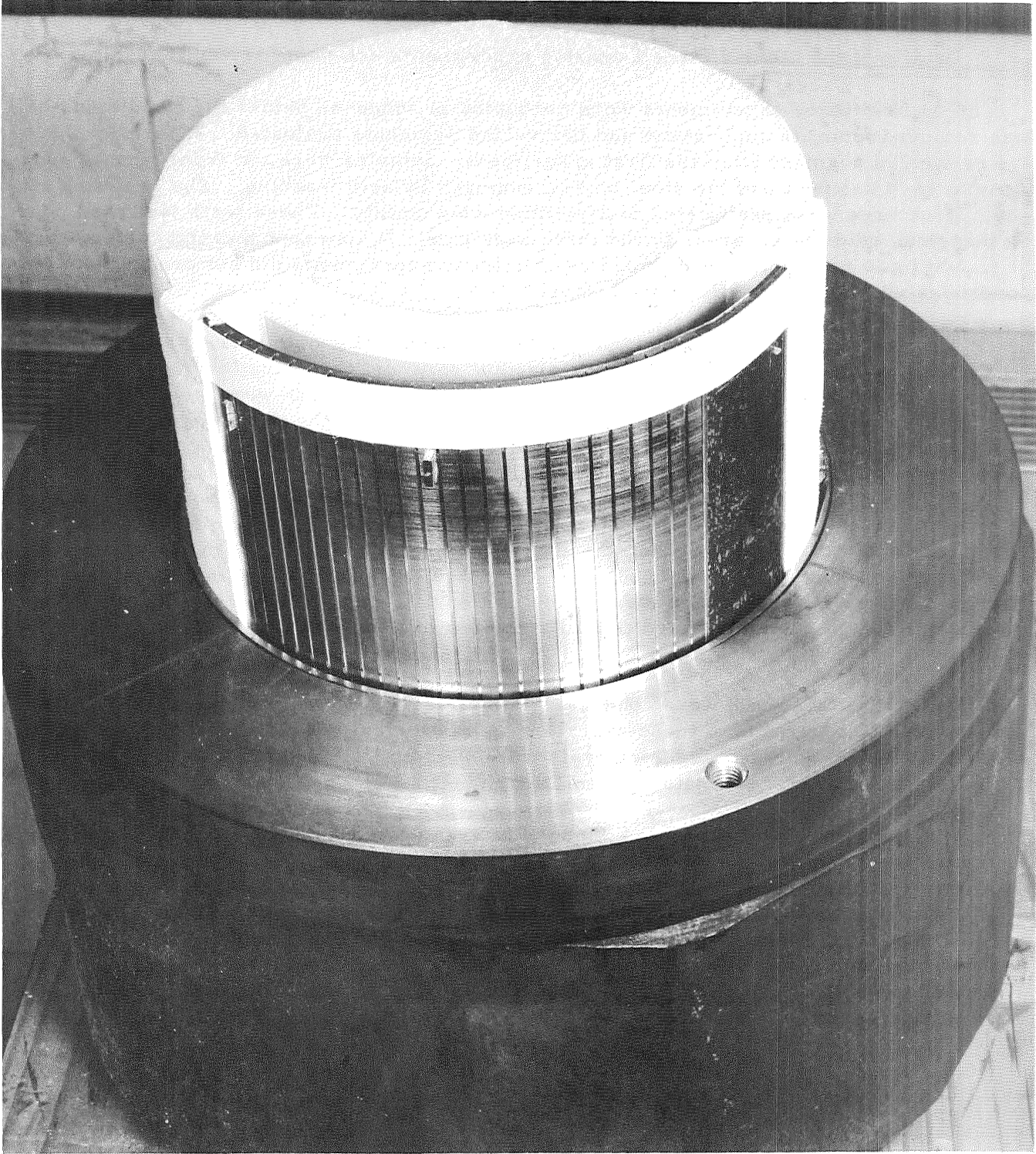
FIGURE 18. PARTIALLY ASSEMBLED SETUP FOR EXPLOSIVELY WELDING A 90-DEGREE RIB-TOOLING SEGMENT TO A SIMULATED SHELL
