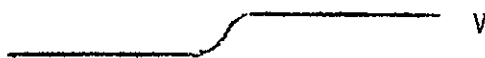
(b.) Potential energy of a negative charge at a \text{Cu}_2\text{S} - \text{Cu}_{1.96}\text{S} interface.
