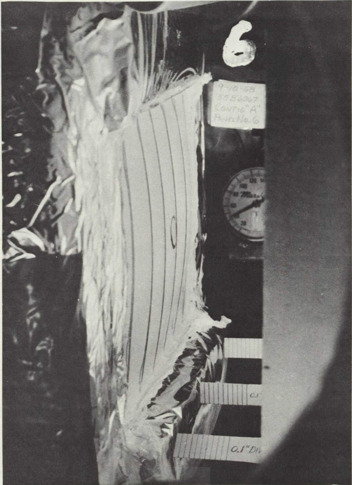
Figure 8-12. Specimen Panel A6 Showing Maximum Blister Formation -- Back Face of Panel at LH 2 Temperature for 2 Hours Before Test
