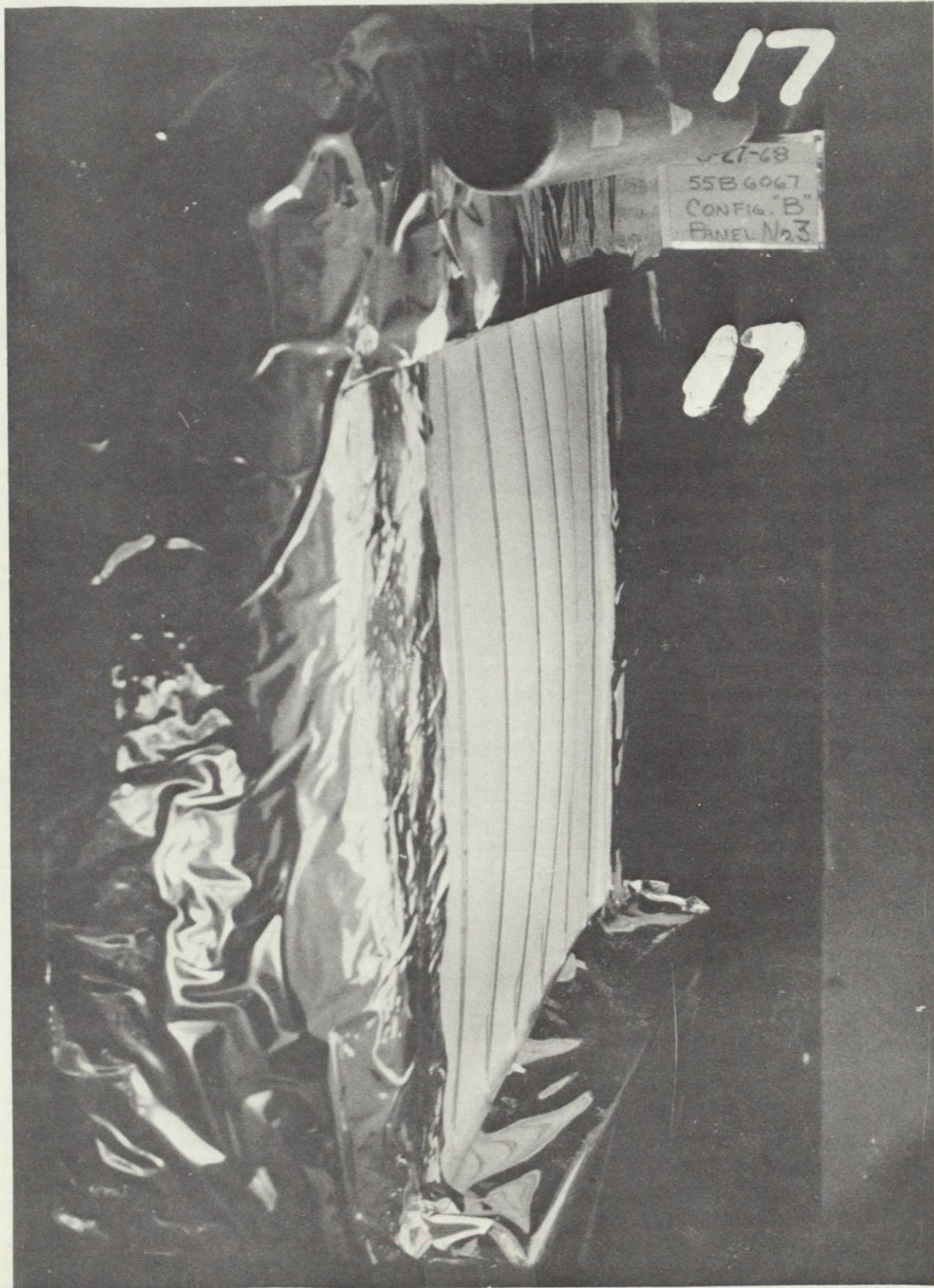
Figure 8-10. Specimen Panel B3 Showing Maximum Blister Formation — Back Face of Panel at LH_2 Temperature for 20 Minutes Before Test
