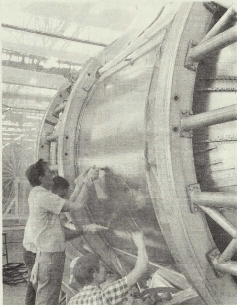
Figure 5-7. Applying Adhesive To The T-9 Tank
