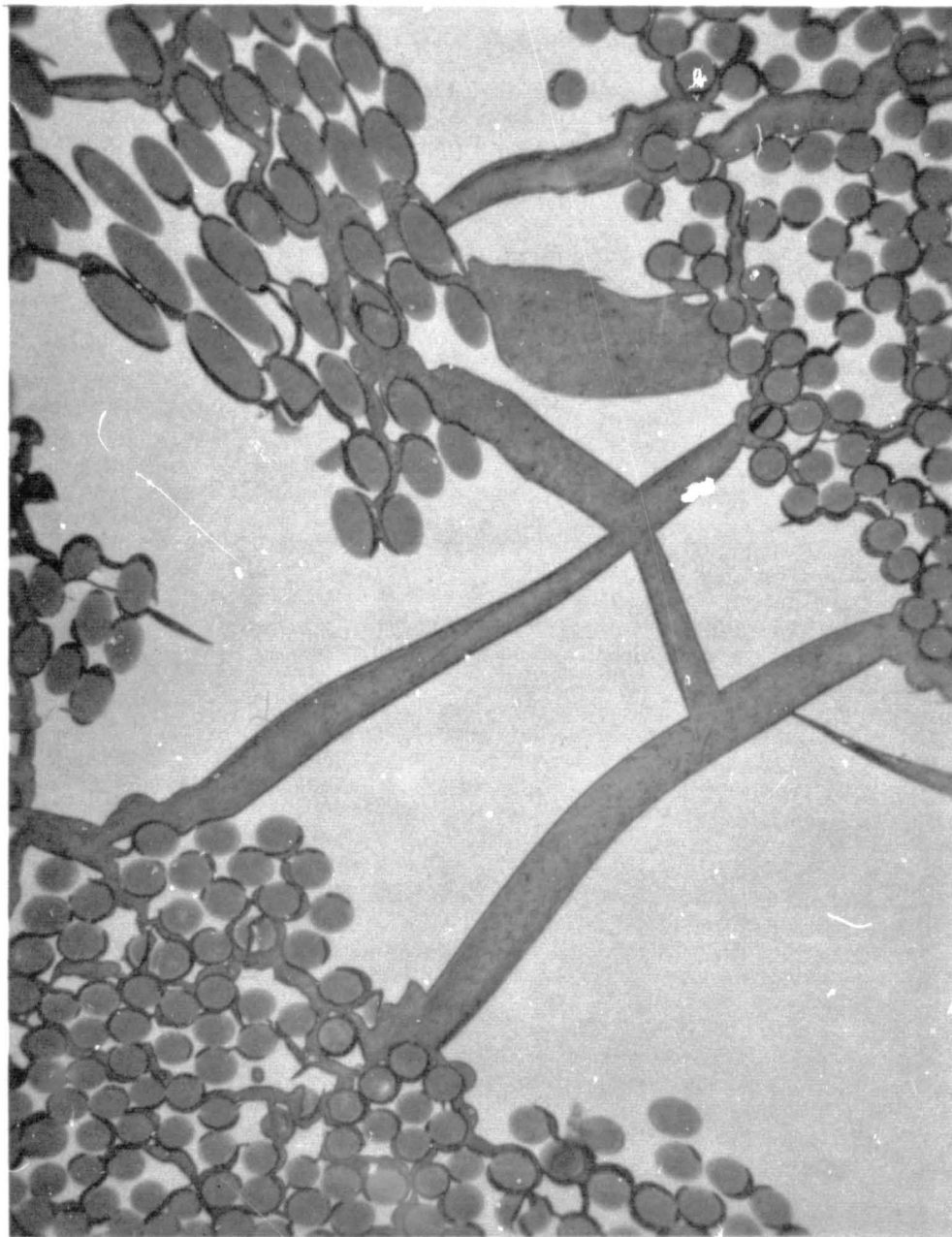
Figure 15 2000°F OVEN-CHARRED SILICA-PHENOLIC MXS-89 CORING (500X MAGNIFICATION)
