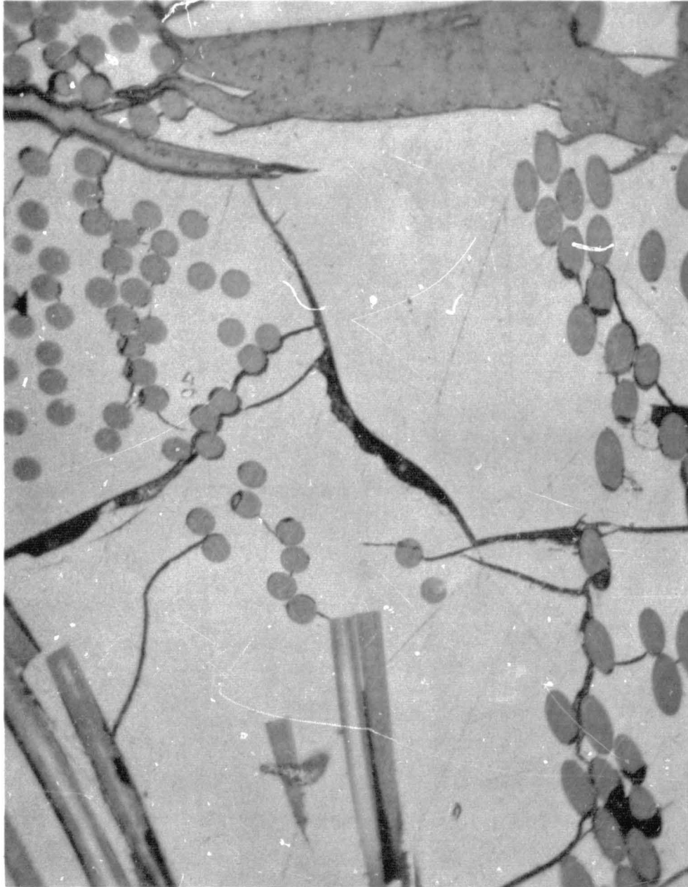
Figure 14 1000°F OVEN-CHARRED SILICA-PHENOLIC MXS-89 CORING (500X MAGNIFICATION)
