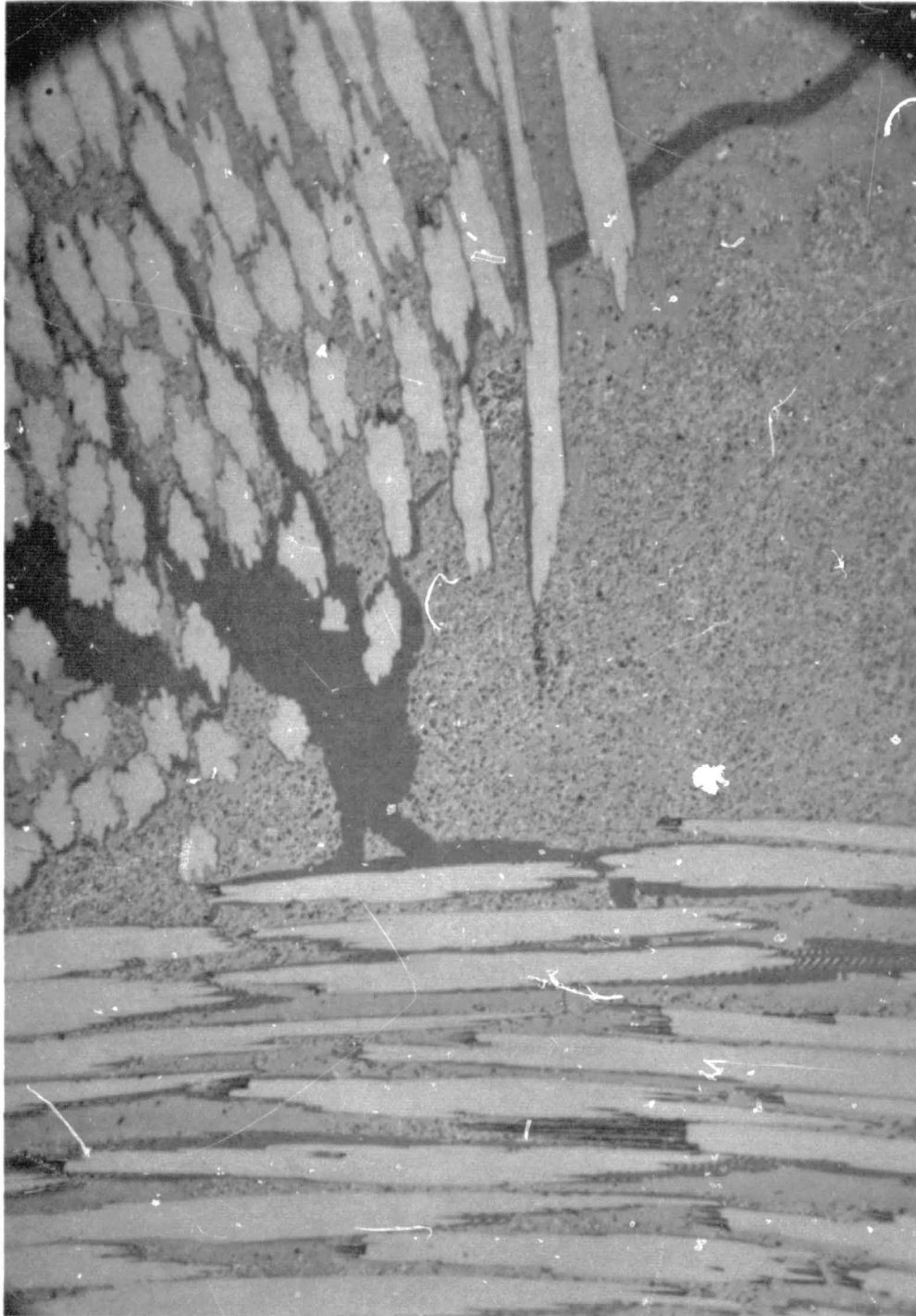
Figure 24 1000°F OVEN-CHARRED GRAPHITE-PHENOLIC MX4501 CORING (500X MAGNIFICATION)
