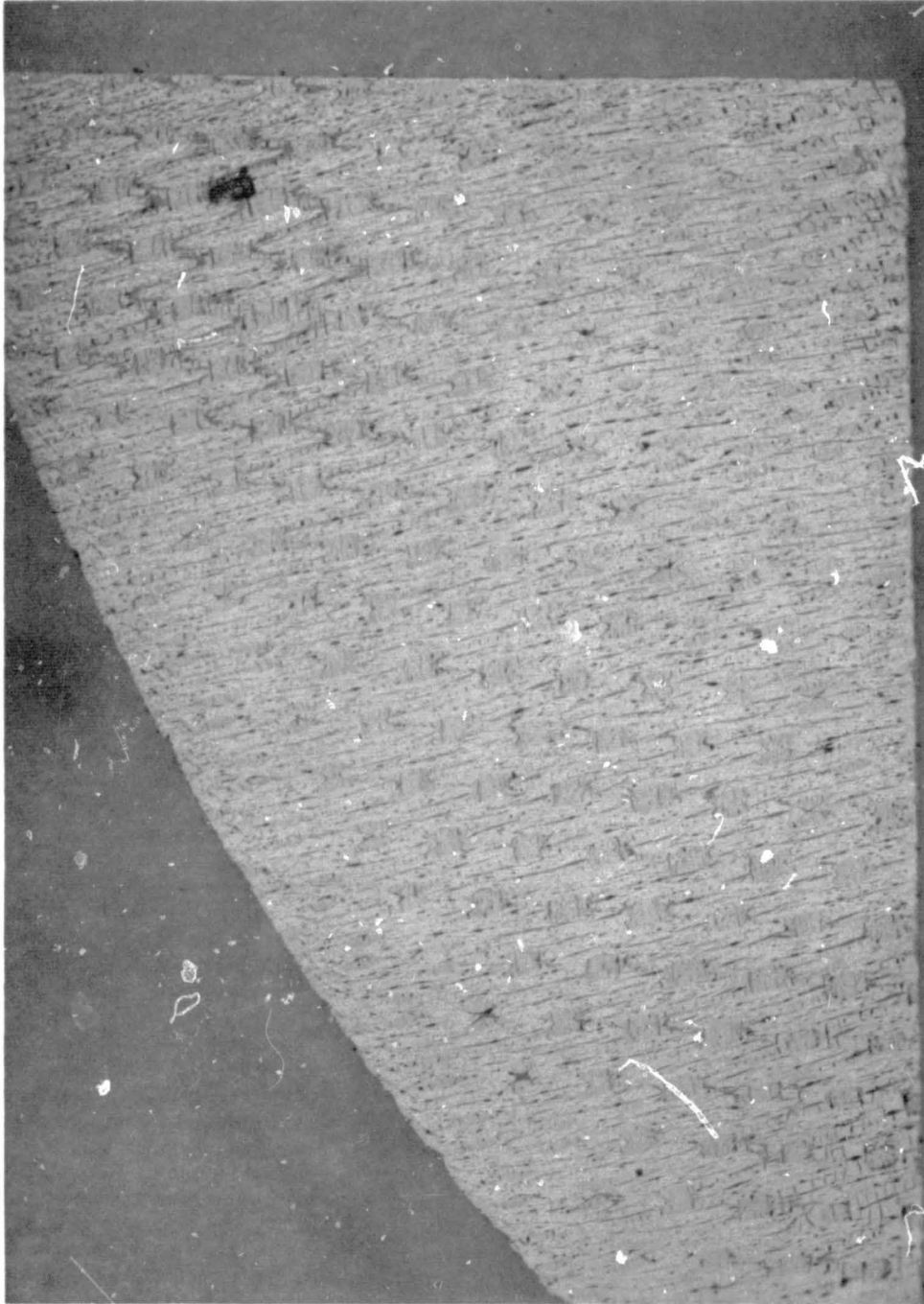
Figure 23 4000°F OVEN-CHARRED GRAPHITE-PHENOLIC MX4501 CORING (5X MAGNIFICATION)
