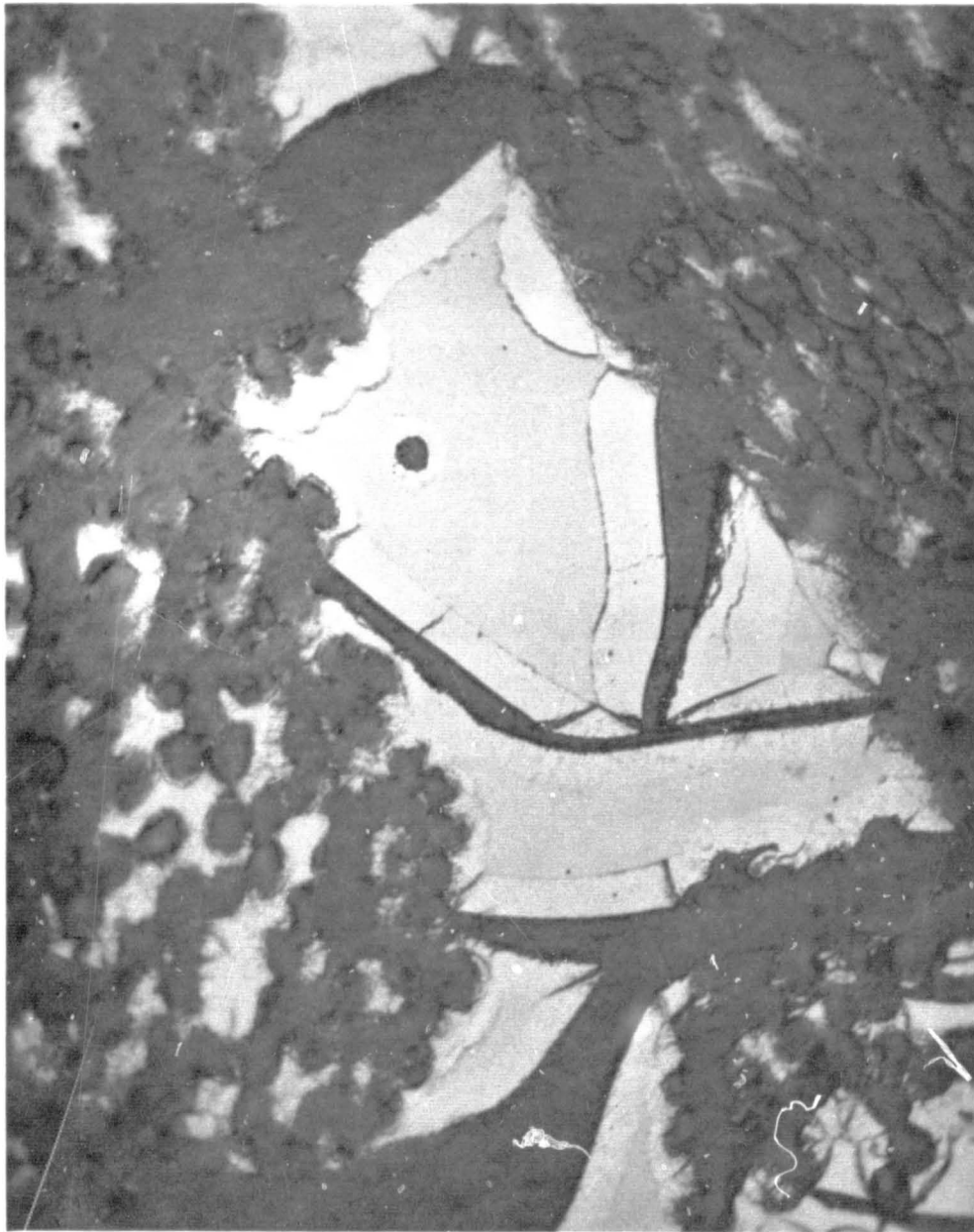
Figure 17 2800°F OVEN-CHARRED SILICA-PHENOLIC MXS-89 CORING (500X MAGNIFICATION)
