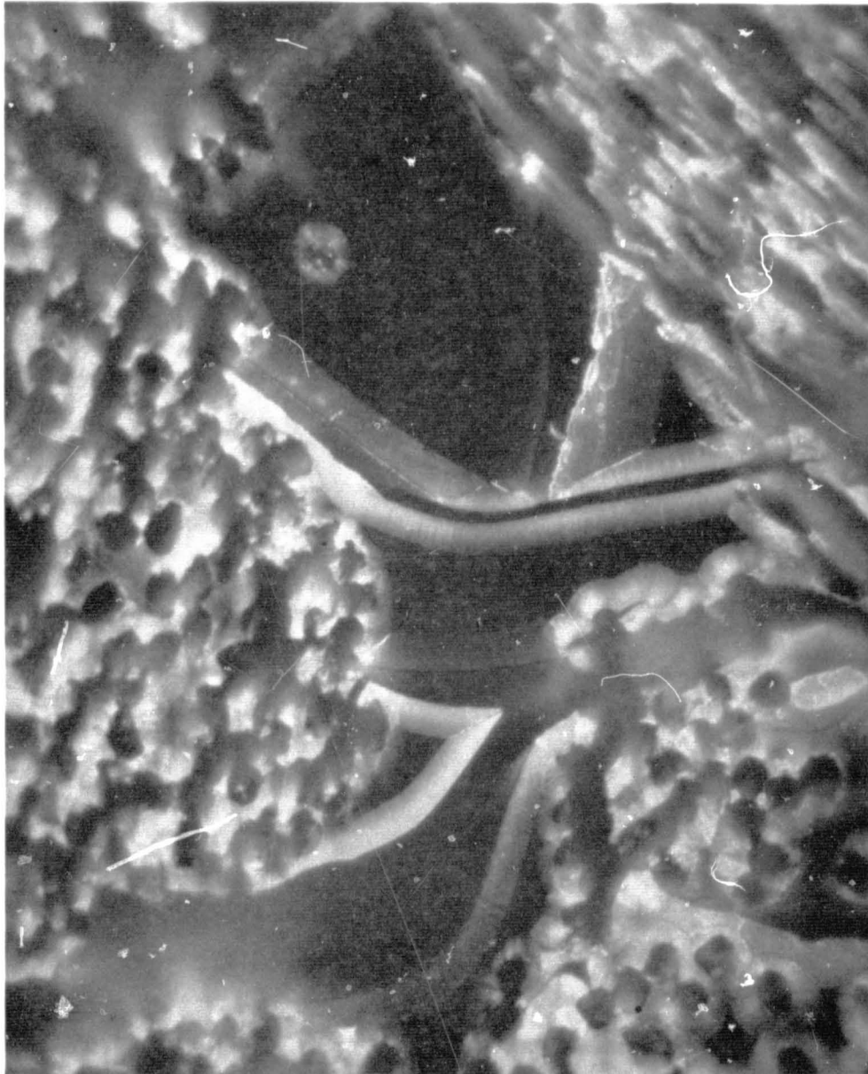
Figure 18 2800°F OVEN-CHARRED SILICA-PHENOLIC MXS-89 CORING (500X MAGNIFICATION -- POLARIZED LIGHTING)
