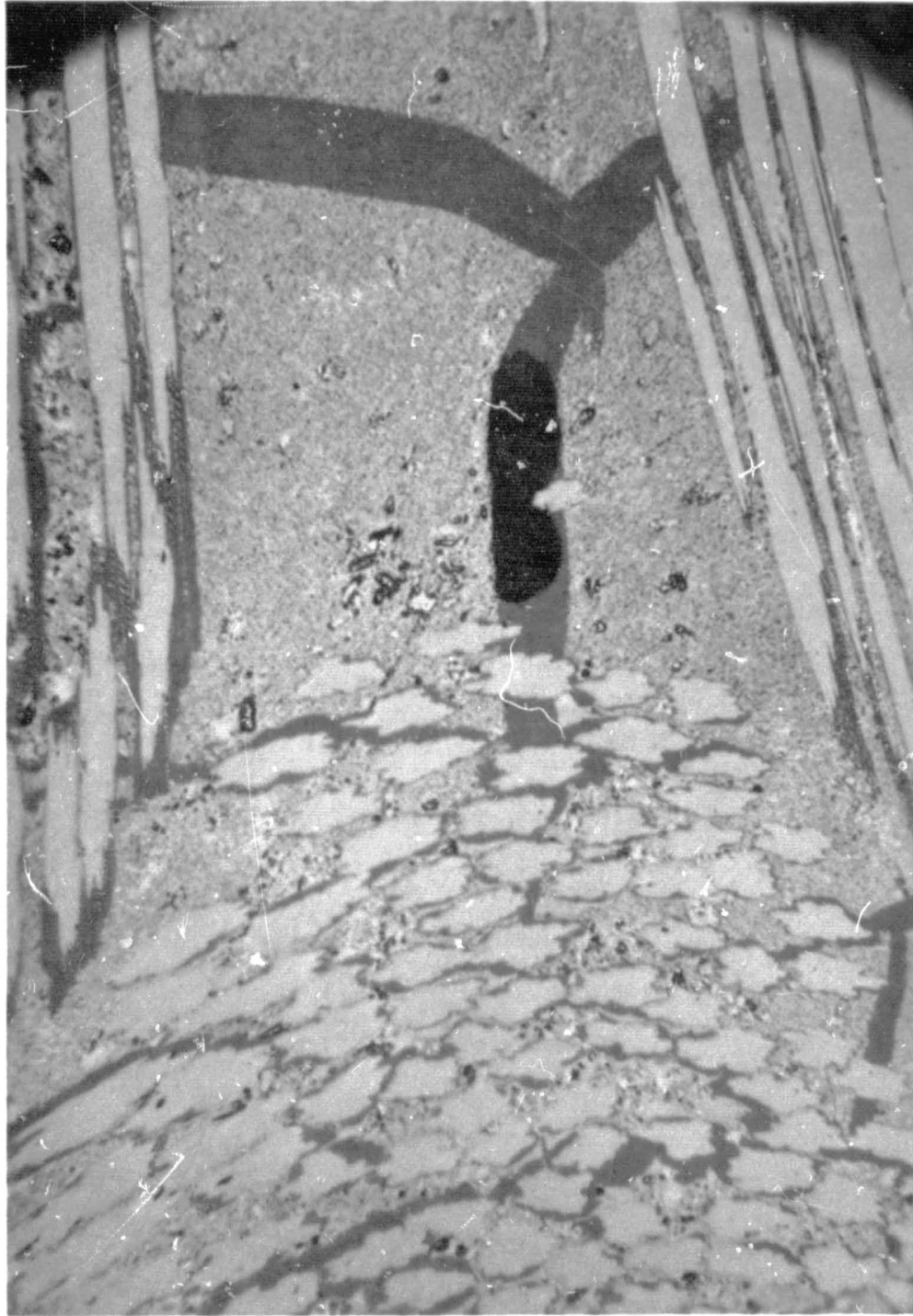
Figure 28 4000°F OVEN-CHARRED GRAPHITE-PHENOLIC MX4501 CORING (500X MAGNIFICATION)
