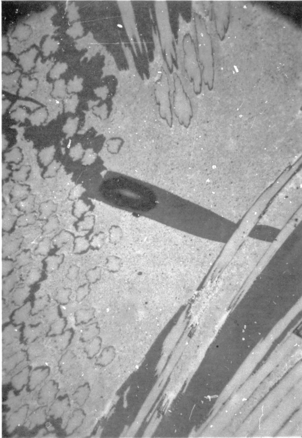
Figure 26 3000°F OVEN-CHARRED GRAPHITE-PHENOLIC MX4501 CORING (500X MAGNIFICATION)
