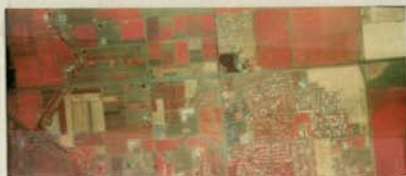
MULTISPECTRAL RENDITION A Green band projected as blue Red band projected as green Infrared band projected as red
