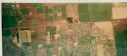
MULTISPECTRAL RENDITION B Green band projected as blue Red band projected as red Infrared band projected as green
