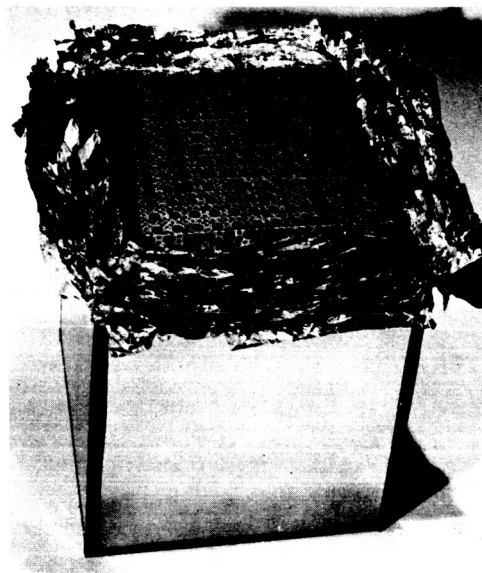
Figure 4-3 THERMALLY CONTROLLED COMPARTMENT MOCKUP for testing ETO penetration consisted of an aluminumized mylar lined box inside outer box. In this photo top sheets of aluminumized mylar removed.
