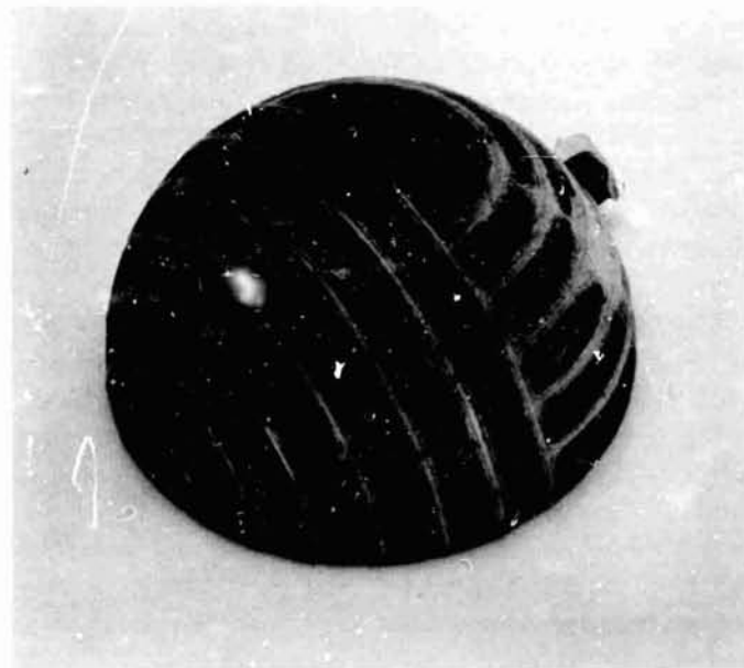
Fig. 1. Folding control pattern of 3/16-in. Teflon rods fused to 18-in. diam hemispherical composite bladder
