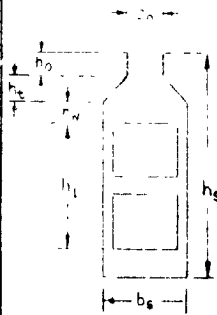
(b) Constant Slot Width (b) For partially closed slots with constant slot width
