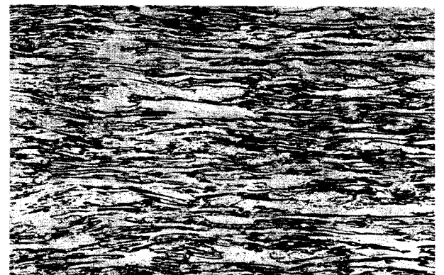
FIG. 7: PHOTOMICROGRAPHS SHOWING ETCHED SECTIONS OF TZM PANCAKE FORGING. 100X, MURAKAMI'S ETCH. AS RECEIVED.
