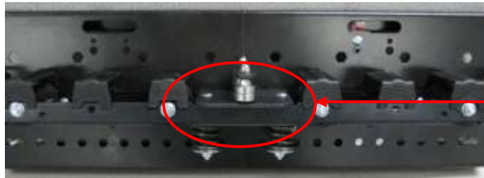
NBC Pressure Pan – spring-to-drive rollers, air-to-accumulate
