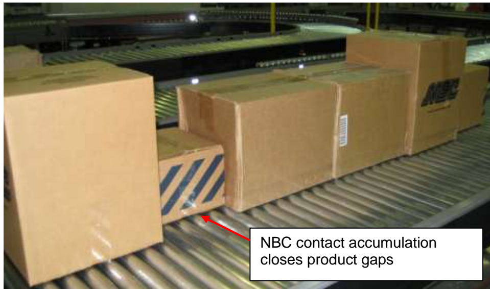
NBC flat belt contact accumulation
