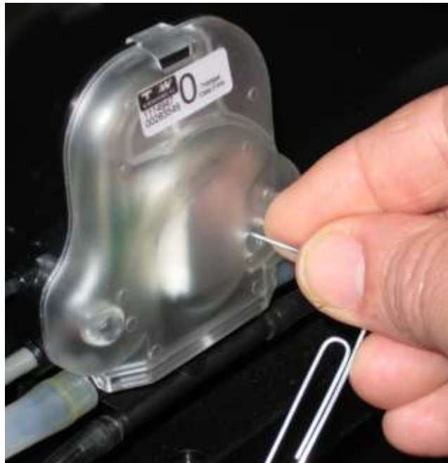
Switching logic modes with paper clip
