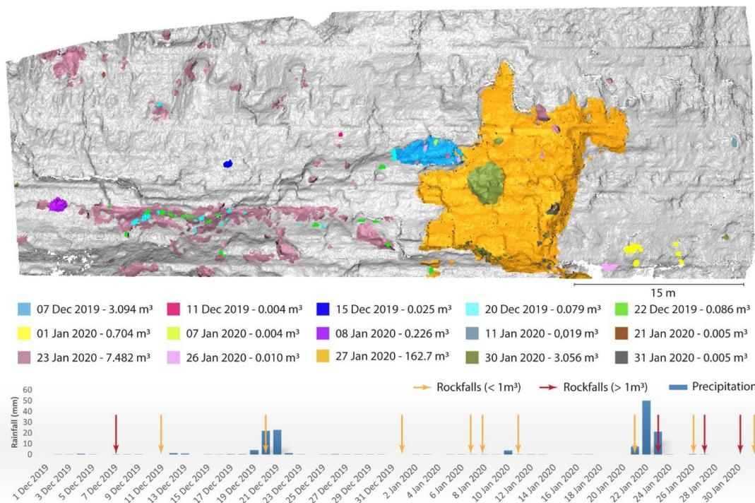
**Figure 7.** Rockfalls occurred on the Puigcercós cliff (NE, Spain) between December 1st and January 31st. Each color corresponds to a different detection date, and the total volume of rockfall per day is calculated. The graph displays the precipitation levels in the area and the days with rockfall activity. Red arrows indicate a total volume detached greater than  $1\text{m}^3$ , while orange arrows indicate a volume less than  $1\text{m}^3$ .
