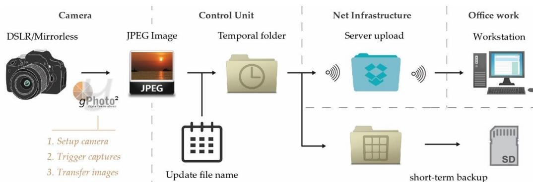
**Figure 3. Illustrative scheme of the workflow implemented in the control unit to communicate with the camera, trigger the camera, send the images remotely, avoiding filling the internal memory of the devices.**
