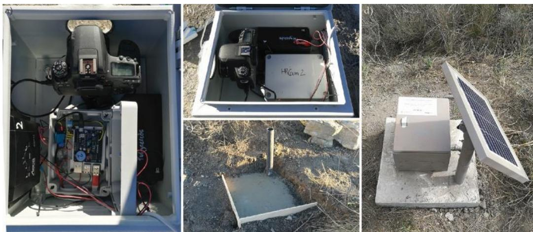
**Figure 1.** Images of the photogrammetric systems installed in the Puigercós site: a and b) Images showing the inside of the photogrammetric unit with part of the connections shown in Figure 3; c) Construction of the concrete base and installation of the PVC pipe for the installation of the photographic units and d) external view of the installed system.
