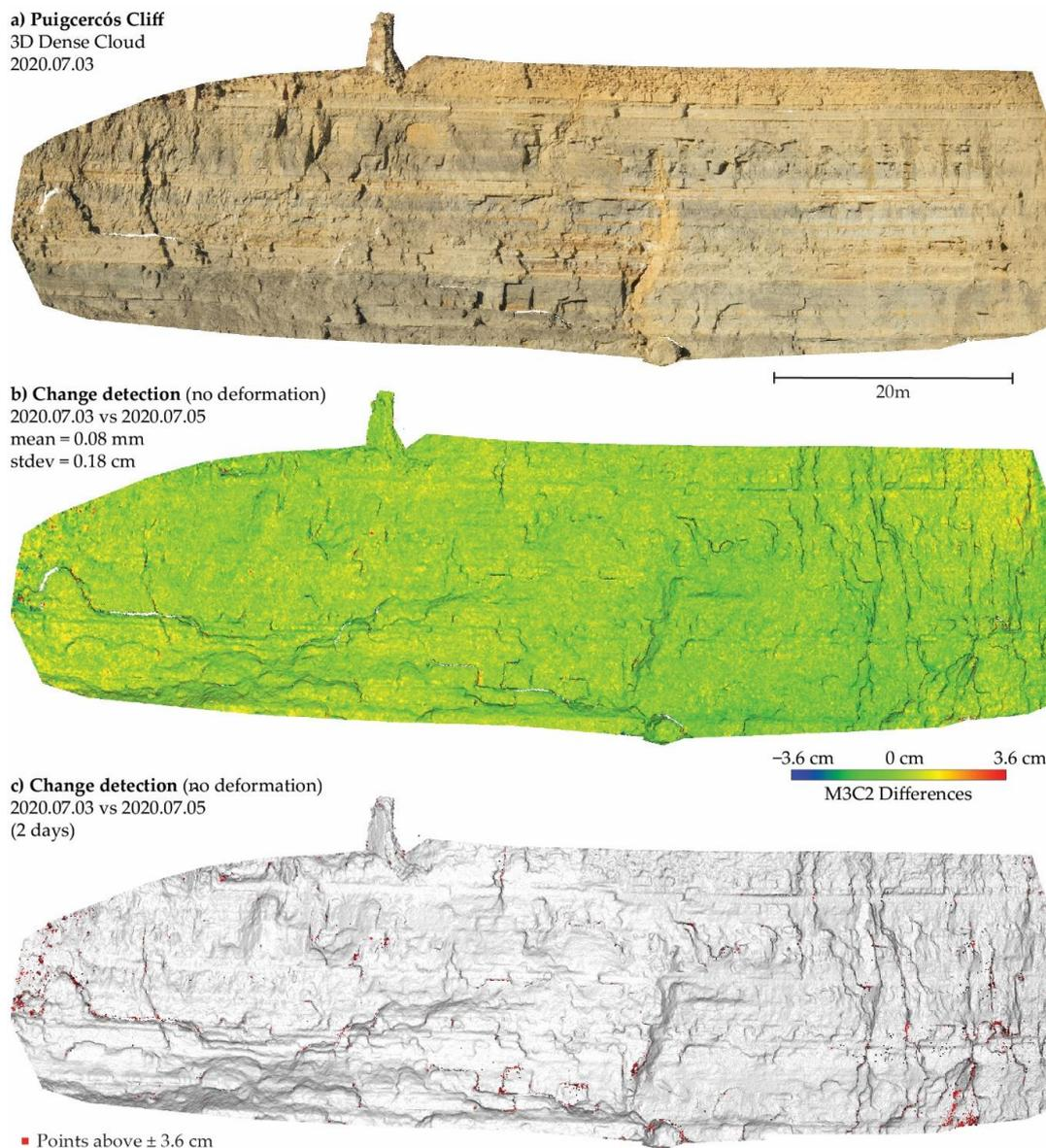
**Figure 5. a) Point cloud obtained with the very high-resolution photogrammetric system installed in Puigercós (obtained with MEMI workflow). b) M3C2 (Lague et al., 2013) comparison of two consecutive days (no expected deformation). c) Same comparison than in b) highlighting in red the points with a deformation higher than 0.036 m.**
