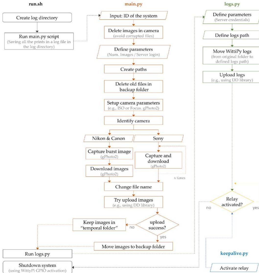
**Figure 4.** Structured flowchart of the open-source codes distributed in the repository of this publication. In grey, the startup code "run.sh", in orange the main code "main.py", in green the code "logs.py" and in blue, the code "keepalive.py" that avoid the shutdown process.
