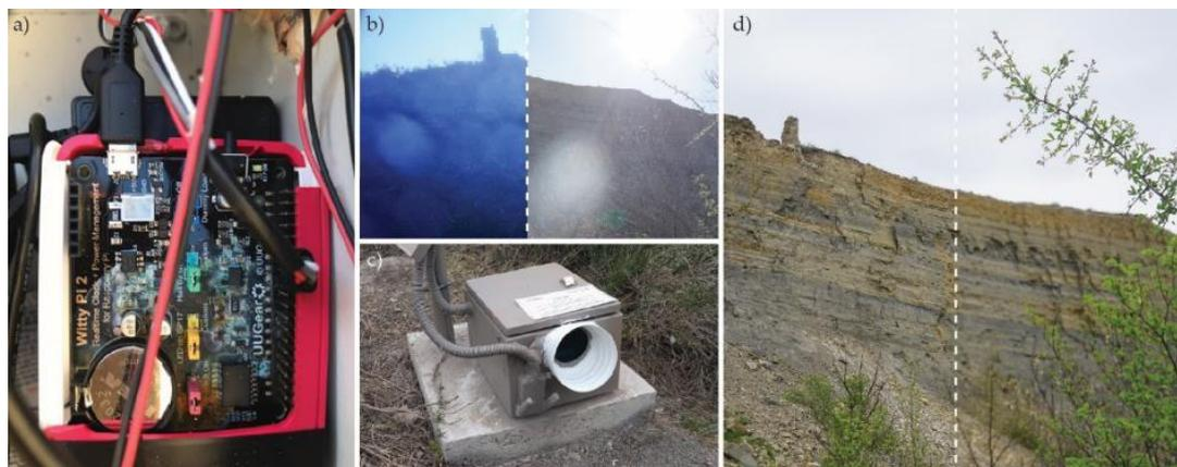
**Figure 8.** Limitations of the high-quality system: a) Rust on the control unit due to water infiltration; b) Image defects due to not incorporating a lens hood. Left: Water drops in the filter glass. Right: lens flare due to the sun's rays; c) Incorporation of the lens hood to avoid the defects shown in b) and the external Wi-Fi antenna; d) Problem due to automatic focus. Left: image with the focus on the cliff. Right: image with the focus on the vegetation in the foreground.
