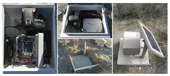
Figure 1. Images of the photogrammetric systems installed in the Puigcercós site: a and b) Images showing the inside of the photogrammetric unit with part of the connections shown in Figure 3; c) Construction of the concrete base and installation of the PVC pipe for the installation of the photographic units and d) external view of the installed system.
