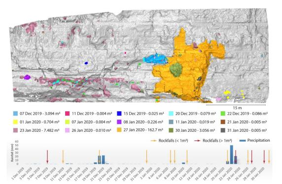
Figure 7. Rockfalls occurred on the Puigcercós cliff (NE, Spain) between December 1st and January 31st. Each color corresponds to a different detection date, and the total volume of rockfall per day is calculated. The graph displays the precipitation levels in the area and the days with rockfall activity. Red arrows indicate a total volume detached greater than 1m<sup>3</sup>, while orange arrows indicate a volume less than 1m<sup>3</sup>.
