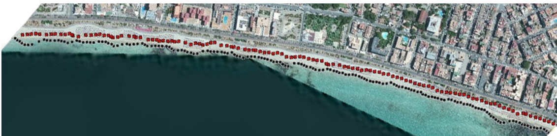
Figure 18. Present-day shoreline position in (black) and landward migration (in red) in the worst case scenario (mean sea level rise under RCP85 and extreme wave conditions) by the end of the 21st century in Playa de Palma beach.
