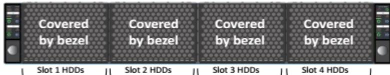
Front HDD bay option enabled configuration for Node CX2560 M4
