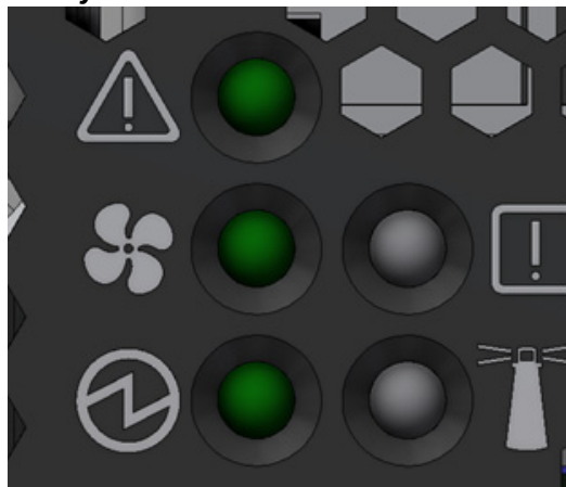
Figure 28: System Status LEDs 5 Minutes After Power On
