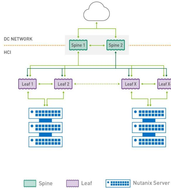
In this example, we use L3 router ports uplinks towards the DC network. The Routing protocol assumed is BGP. Multi-Active Gateway Protocol (MAGP) will be used as the host's (VM's) gateways to communicate with outer networks. Each VLAN must have its own MAGP instance to be able to communicate with other VLANs or external networks. The configuration is done on the leaf switches' level.
