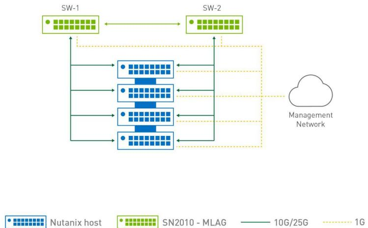
In the diagram that will be used for this guide, there are four Nutanix Nodes that are connected using an Active-Active LACP bond to a pair of NVIDIA SN2010 switches that are configured in MLAG.
