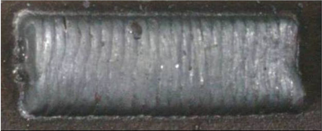
Figure 32. Methane Weld Specimen 325-8
