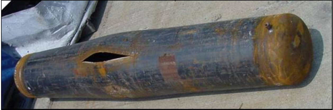
Figure 54. Unbent Pipe Section after Hydrostatic Burst Test
