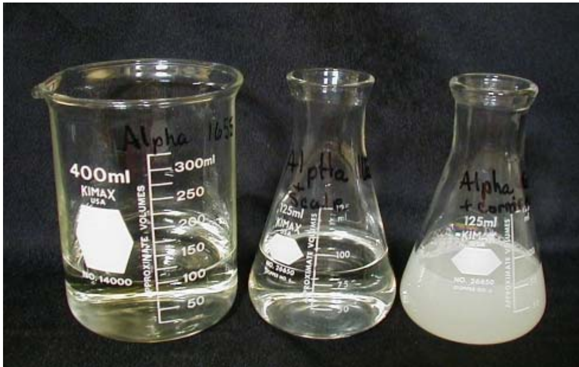
Figure 14. Left to right: Visual observation of Alpha 1655 (30,000 ppm), mixture of Alpha + scale inhibitor (12,600 ppm), and mixture of Alpha + corrosion inhibitor (2,600 ppm).
