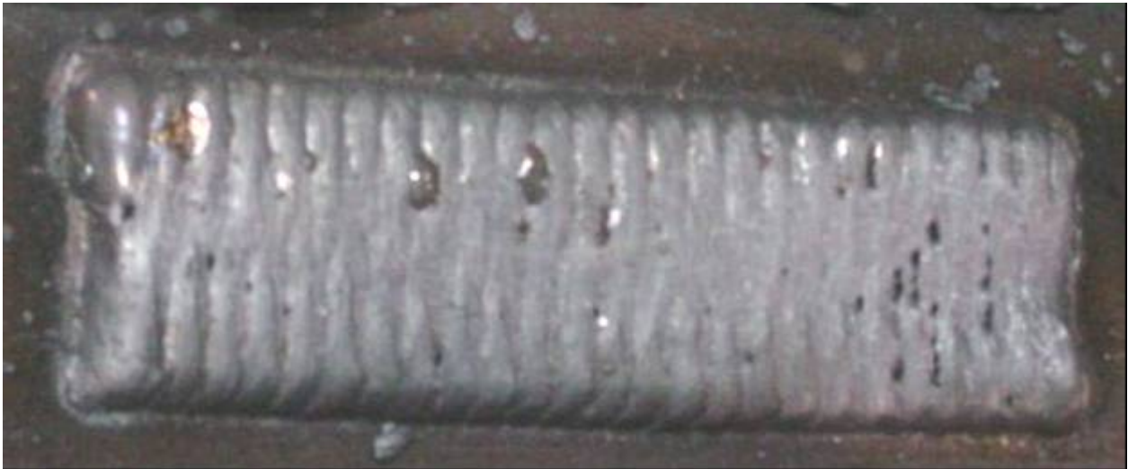
Figure 33. Methane Weld Specimen 325-9
