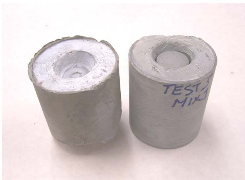
Figure 9. Photograph of MPro specimens, after curing and removal from test vessel (left), showing indentations from transducers, and after coring 1" diameter plug (right), with machined end surfaces, for load frame tests.
