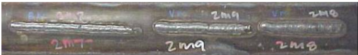
Figure 21. Welds Made in Pressurized Methane - Appearance from OD
