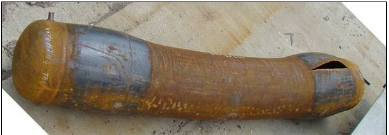
Figure 55. Bent Pipe Section after Hydrostatic Burst Test
