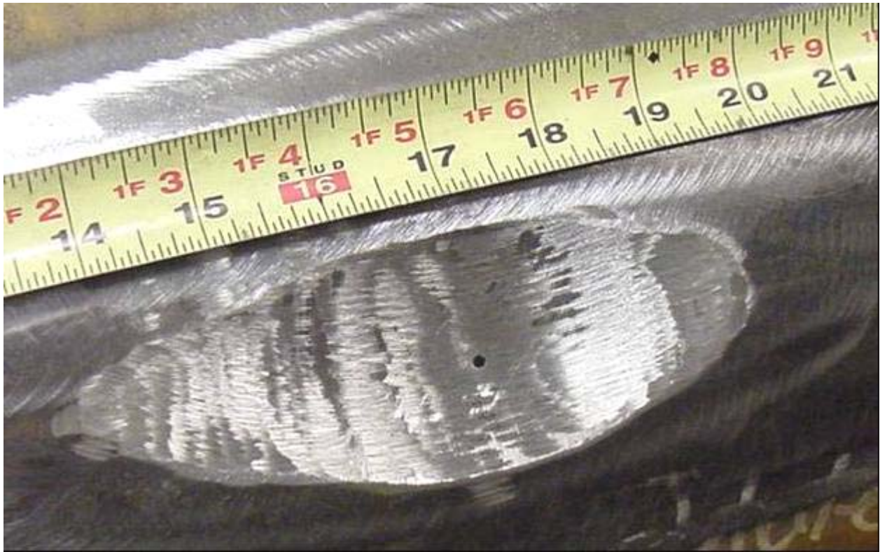
Figure 52. Simulated Corrosion with Through Hole
