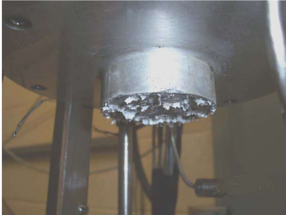
Figure 6. Particulate material deposited on the upper end platen, presumably from within an aqueous layer during several days in which the cement specimen was in the vessel.
