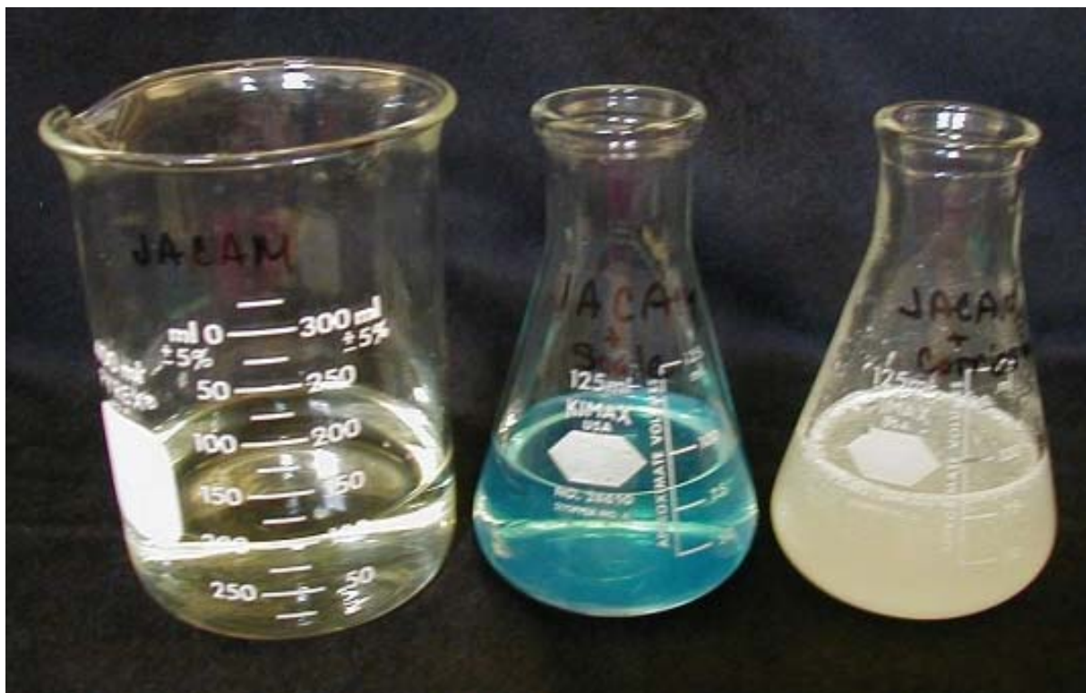
Figure 12. Left to right: Visual observation of JACAM (30,000 ppm), mixture of JACAM + scale inhibitor (9,460 ppm), and mixture of JACAM + corrosion inhibitor (1,300 ppm).
