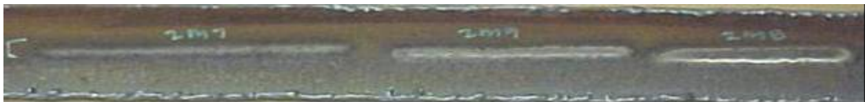
Figure 22. Welds Made in Pressurized Methane - Appearance from ID
