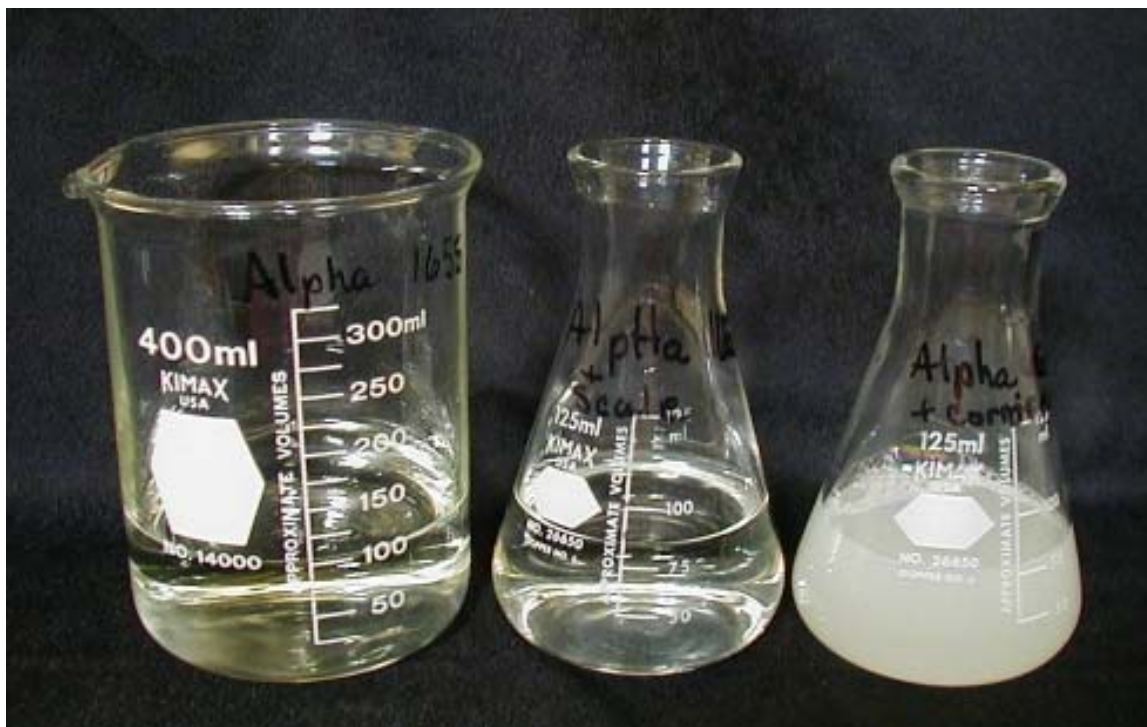
Figure 15. Left to right: Visual observation of mixture of Alpha 1655 (30,000 ppm), mixture of Alpha + scale inhibitor (12,600 ppm), and Alpha + corrosion inhibitor (2,600 ppm).
