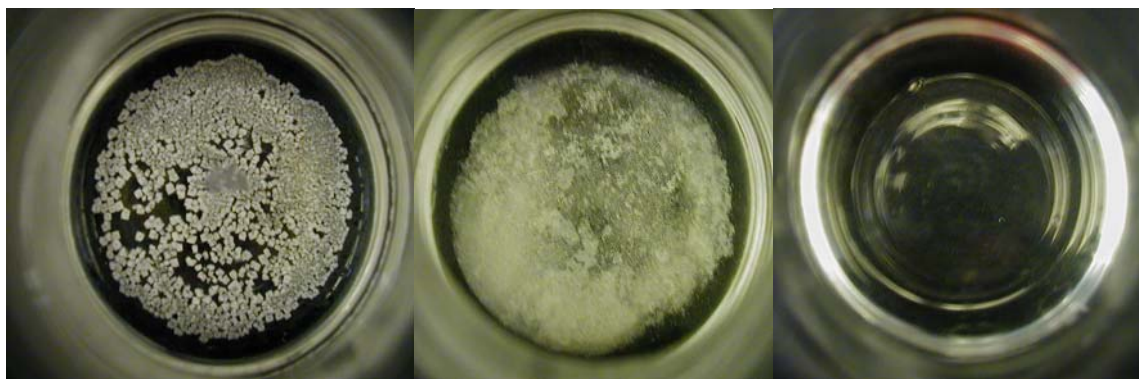
Figure 3. Three views of NaCl brine solutions; left to right, brine solution with no inhibitor, brine solution with 0.01% of \text{Fe}(\text{CN})_6 inhibitor, and brine solution with 0.05% \text{Fe}(\text{CN})_6 inhibitor.
