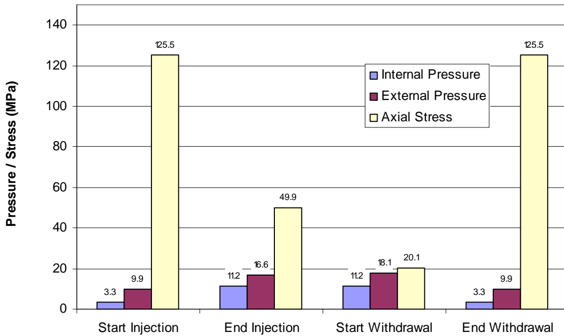
Figure 6-15. Load Steps for the Connection in Salt Cavern Well No. 1 at a Depth of 567 Meters (1,860 Feet).
