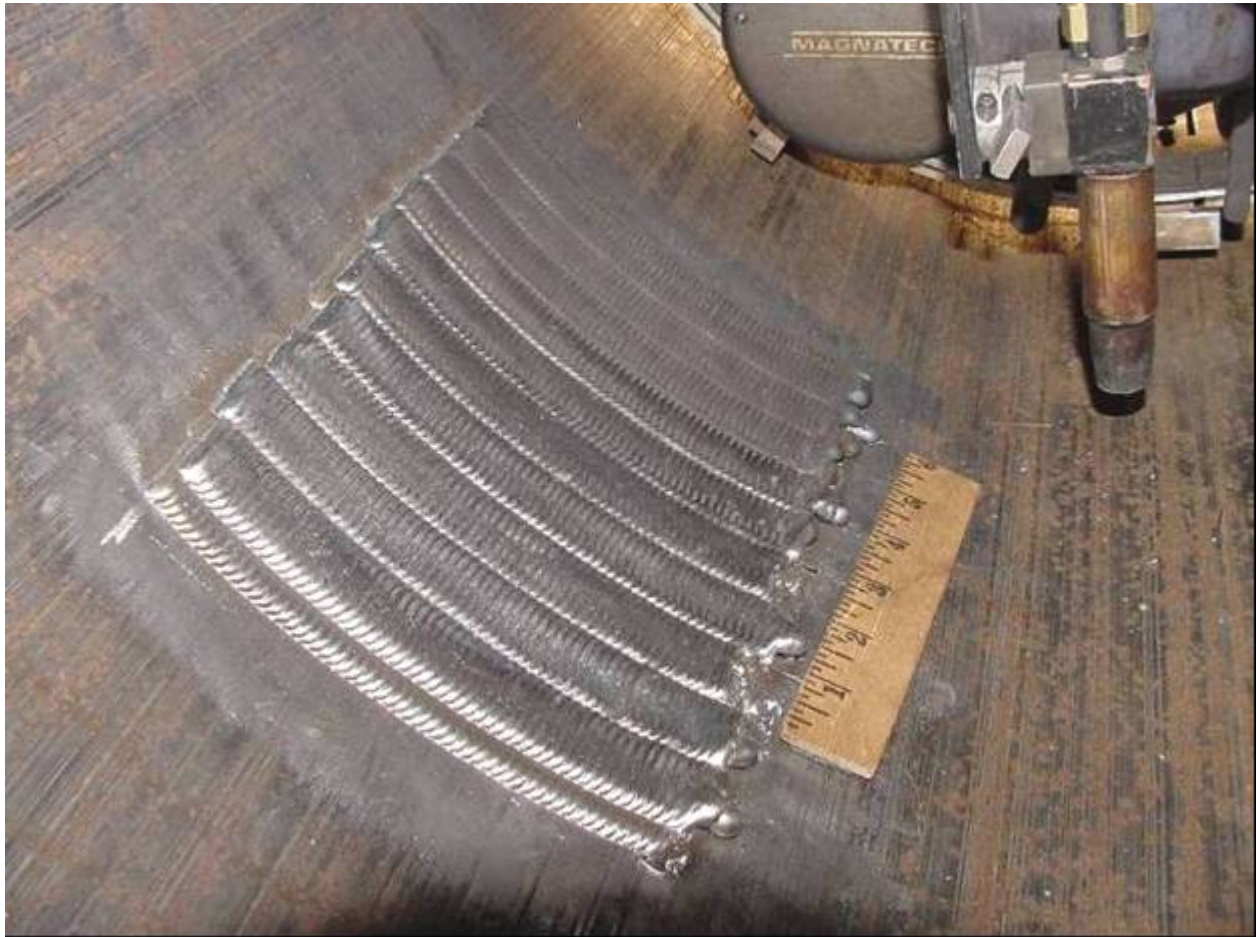
Figure 34. Test 01 Finished Patch Type Weld Repair
