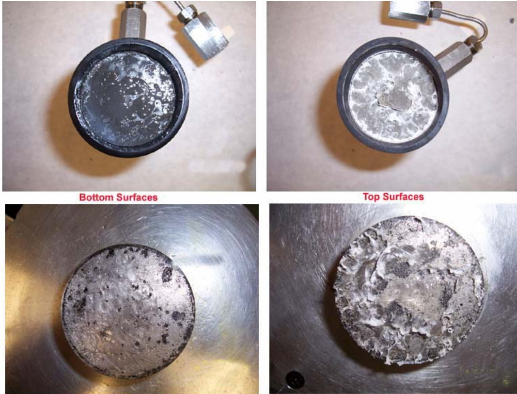
Figure 7. Post test photographs of top (right side) and bottom (left side) surfaces of test specimen (top) and end platens (bottom).
