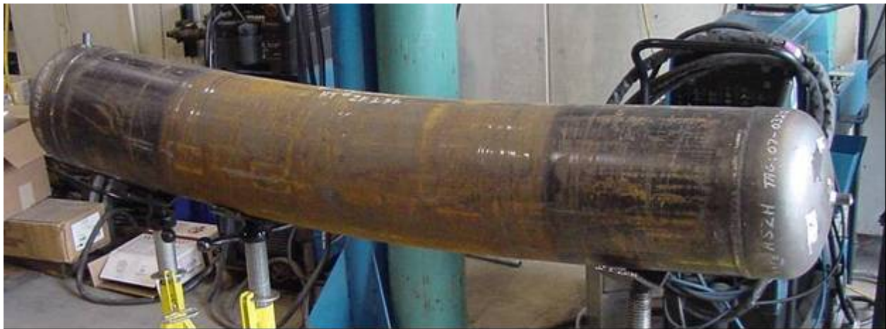
Figure 51. Bent Pipe Section for Helical Strap Repair Feasibility
