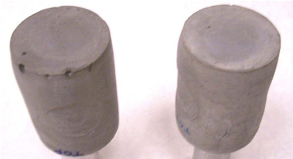
Figure 41. Photographic comparison of post-test Specimen 10 (left side) and 11 (right side), showing greater porosity in Specimen 10.
