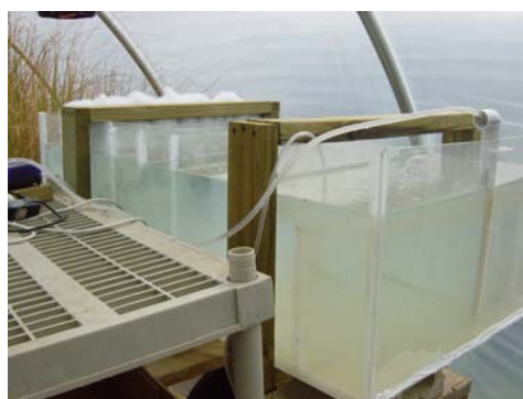
Figure 27: Newly constructed Oil/Water Separator used in Experiment 4.
