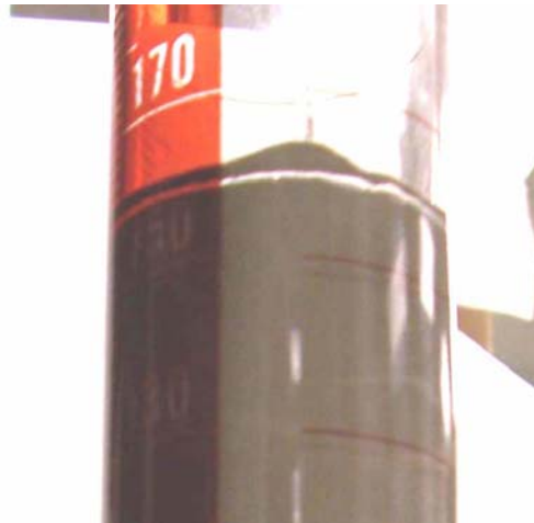
Figure 4. Side view of a graduated cylinder (250 ml) filled with cement slurry, after curing overnight. The white line around the circumference at the top of the cement column delineates the zone initially occupied by water expelled from the cement, and later re-absorbed
