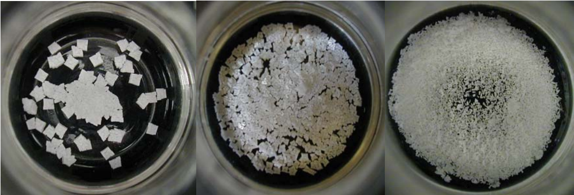
Figure 6. Left to right: precipitate from supersaturated NaCl solution, precipitate from supersaturated NaCl solution with Ca hardness, and precipitate from supersaturated NaCl solution with Ca hardness and salt inhibitor.
