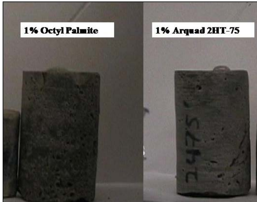
Figure 16. Water drops on treated dolomite are similar to contact angles shown in Fig. 14.
