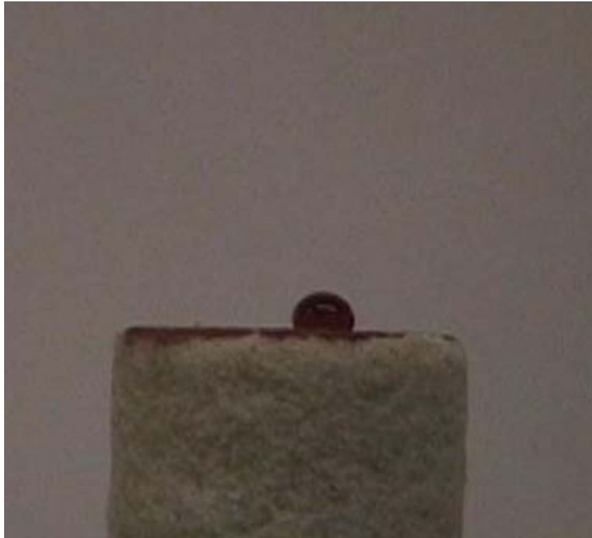
Figure 15. Water drop contact angle on treated sandstone is less than 90^\circ .
