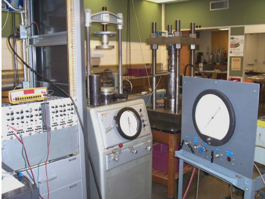
Figure 12. Load frame (center), with ancillary electronics and meters for static deformation tests.
